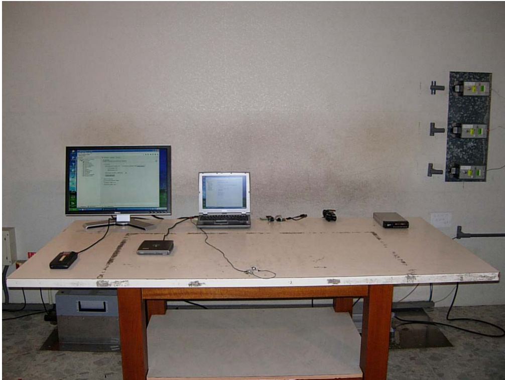
Front View of Conducted Test
