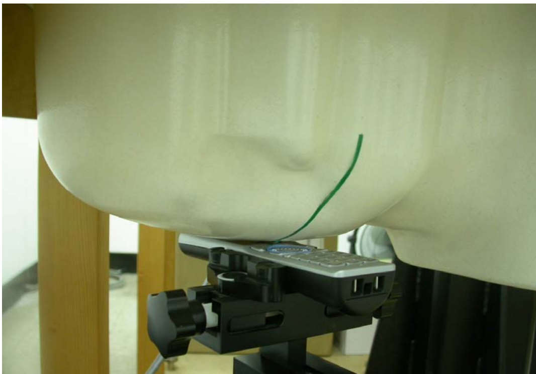
Measurement Position of Right-Tilt (RT) with Handset
