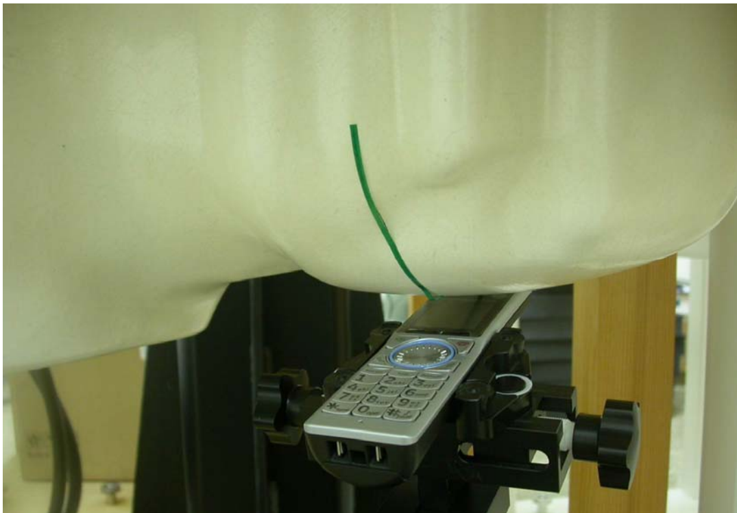
Measurement Position of Left-Cheek (LC) with Handset
