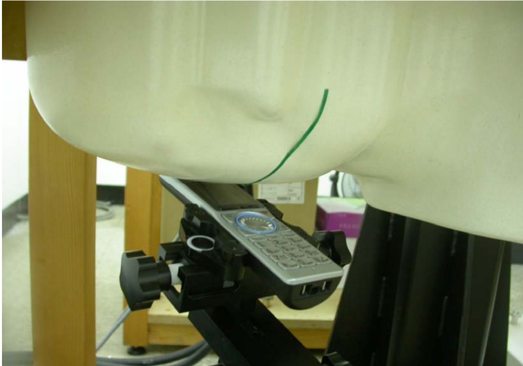
Measurement Position of Right-Cheek (RC) with Handset
