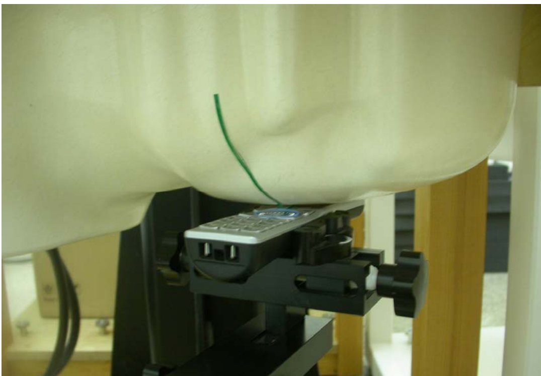
Measurement Position of Left-Tilt (LT) with Handset
