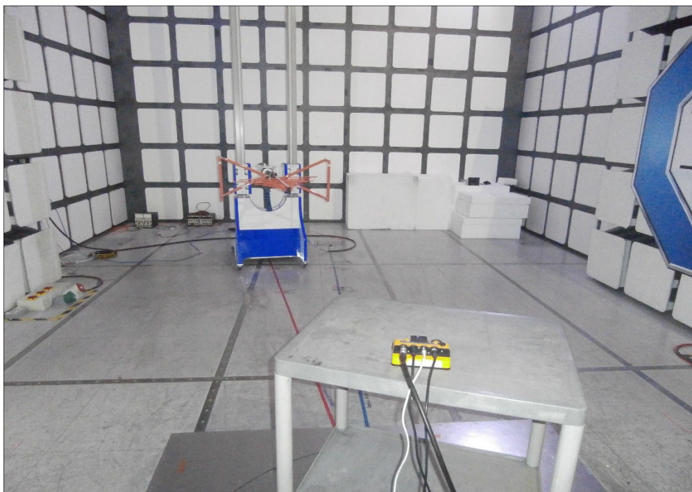
Figure 6 - Test Setup - Radiated Emissions 30 MHz to 1 GHz
