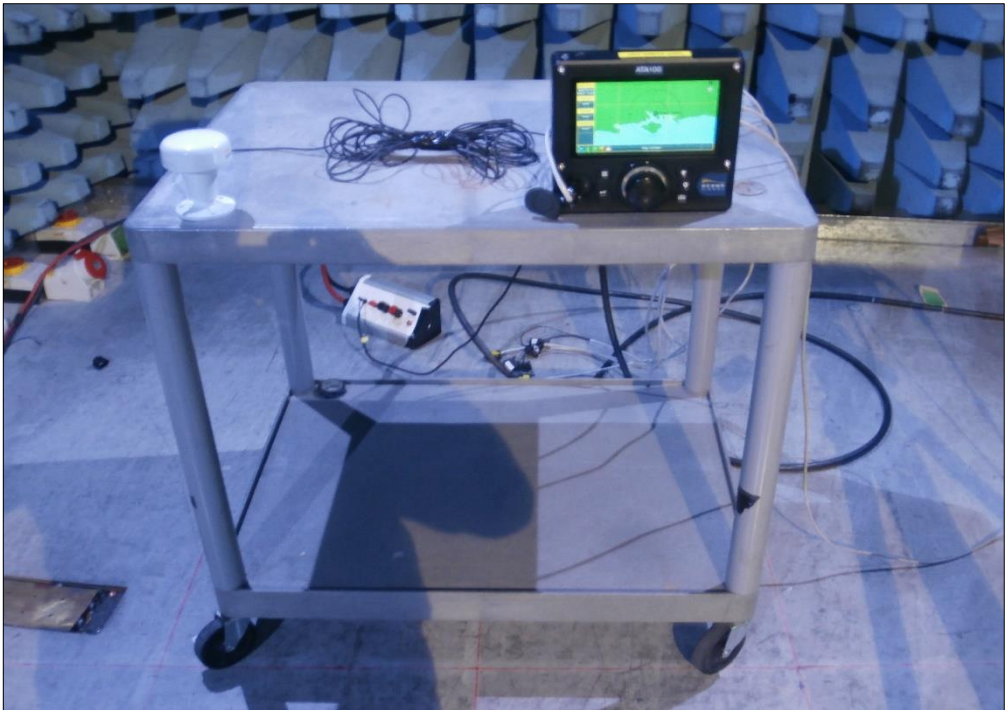
Figure 13 - Test Setup - Immunity to radiated radio frequencies
