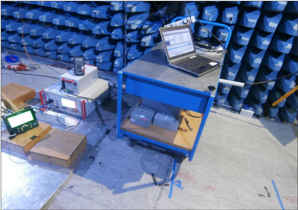
Figure 14 - Test Setup - Immunity to Power Supply Failure
