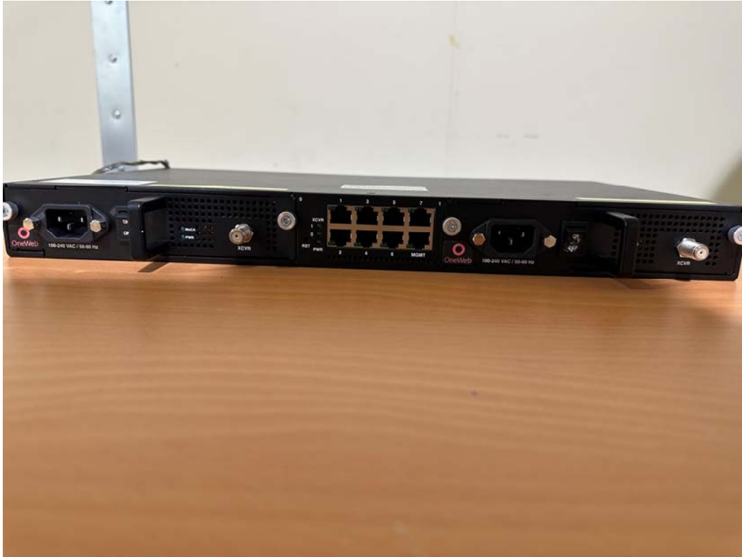
Customer Network Exchange I/O port
