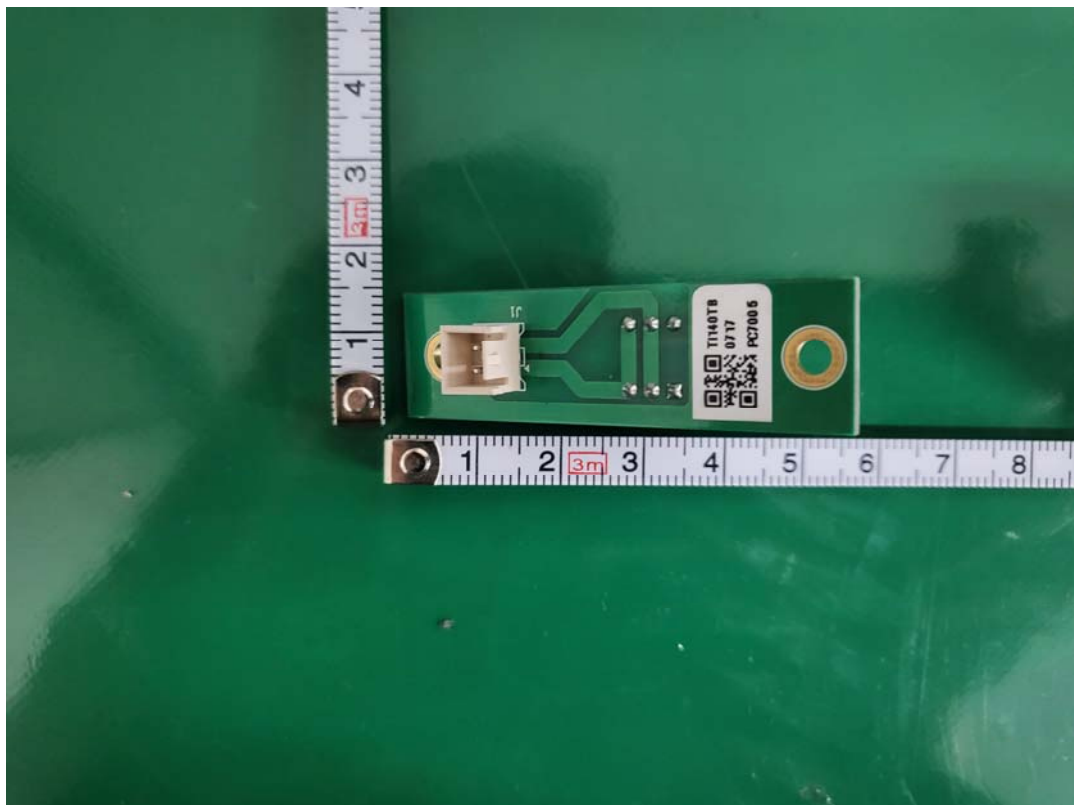
Switch board - Rear
