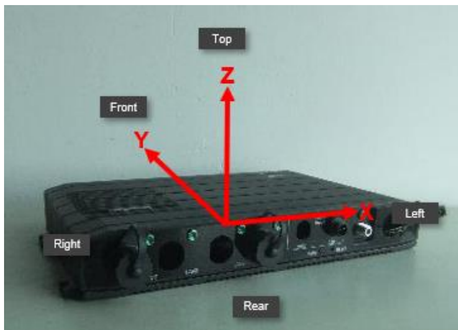
Figure 2: Model N01AZAAA Measurement axes
