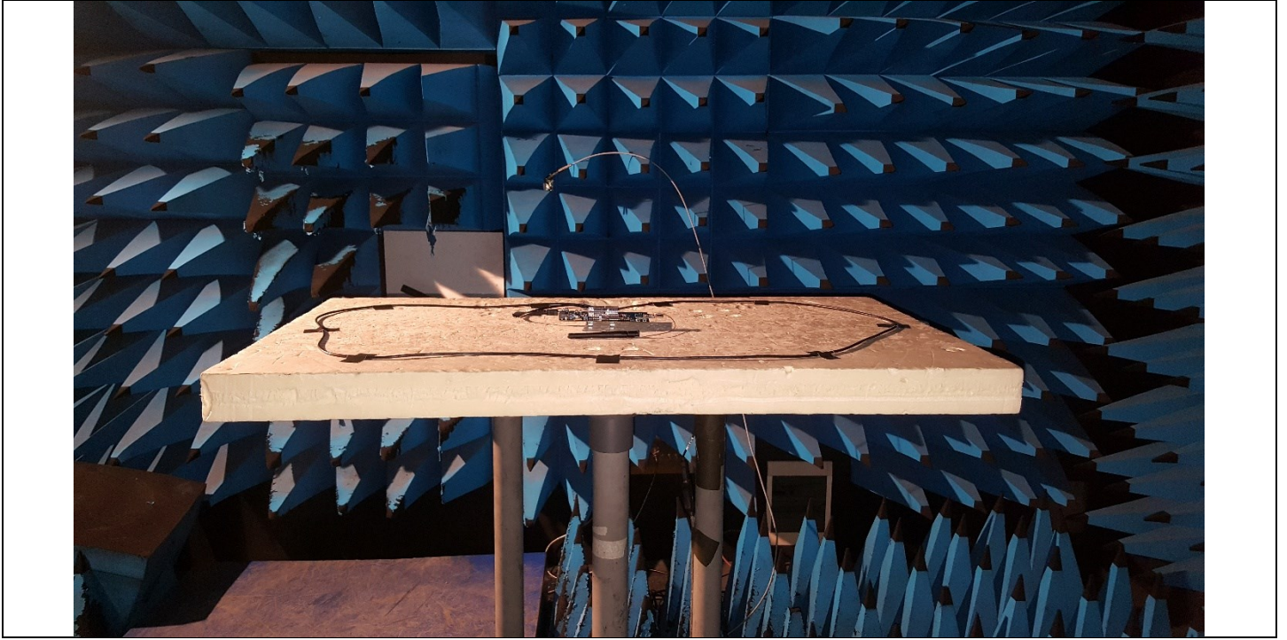
Photograph for Unwanted Emission in restricted frequency bands (M13)
