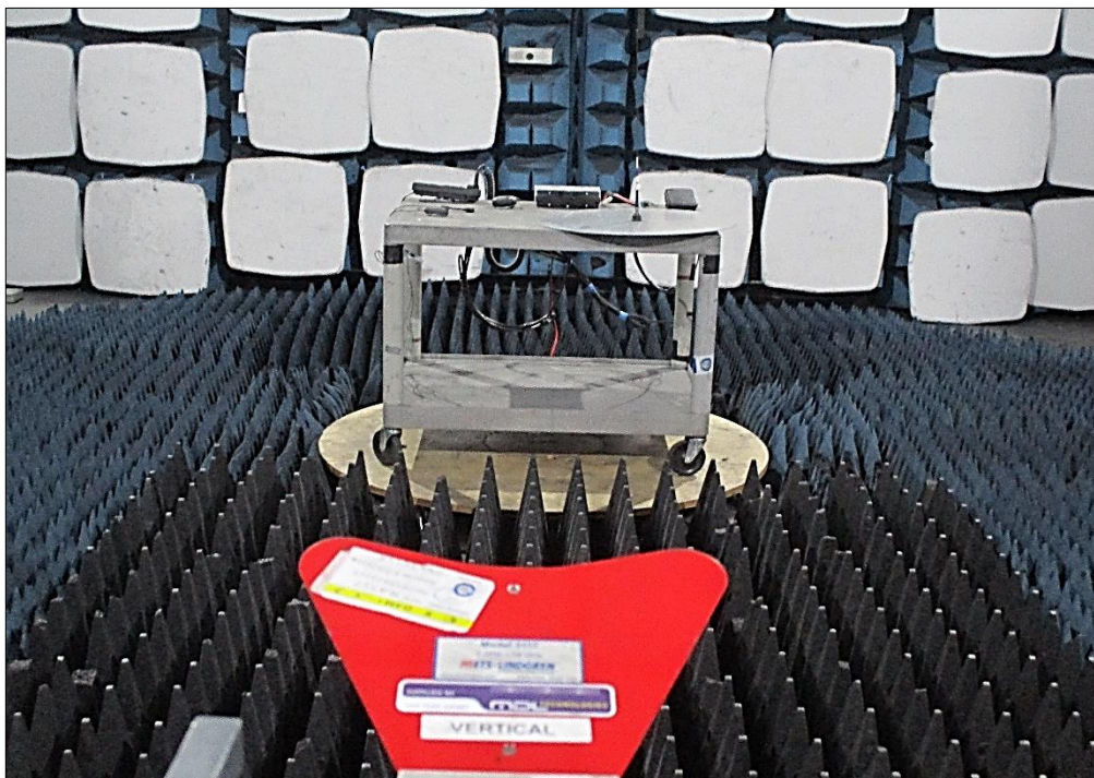
Figure 13 - Test Setup - 1 GHz to 13 GHz
