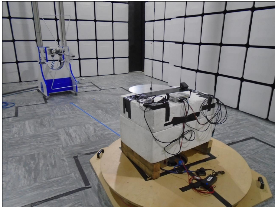
Figure 8 - Test Setup - 30 MHz to 1 GHz
