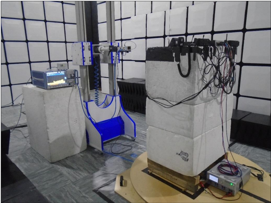
Figure 11 - Test Setup - 18 GHz to 25 GHz
