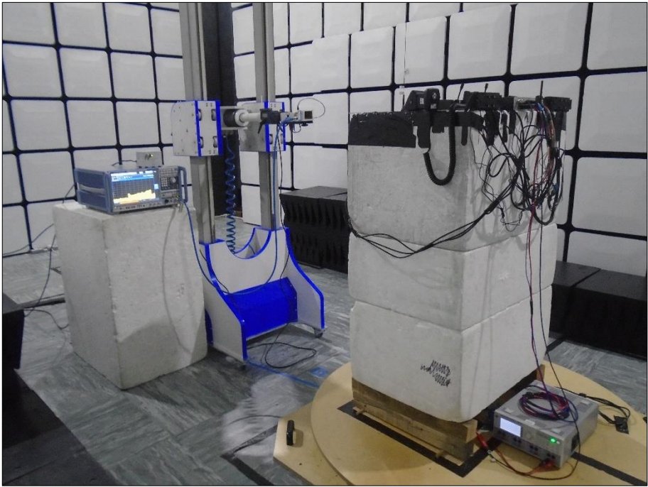
Figure 17 - Test Setup - 18 GHz to 25 GHz
