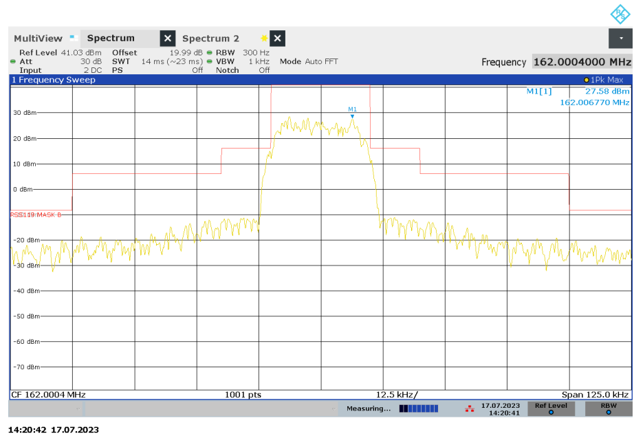
Figure 26 - 162 MHz, Transmitter Mask
