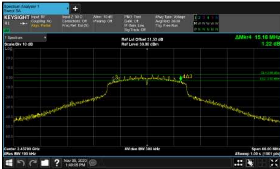
Figure 27 - Core 0 (A) 2437 MHz (CH6) 6 dB Bandwidth
