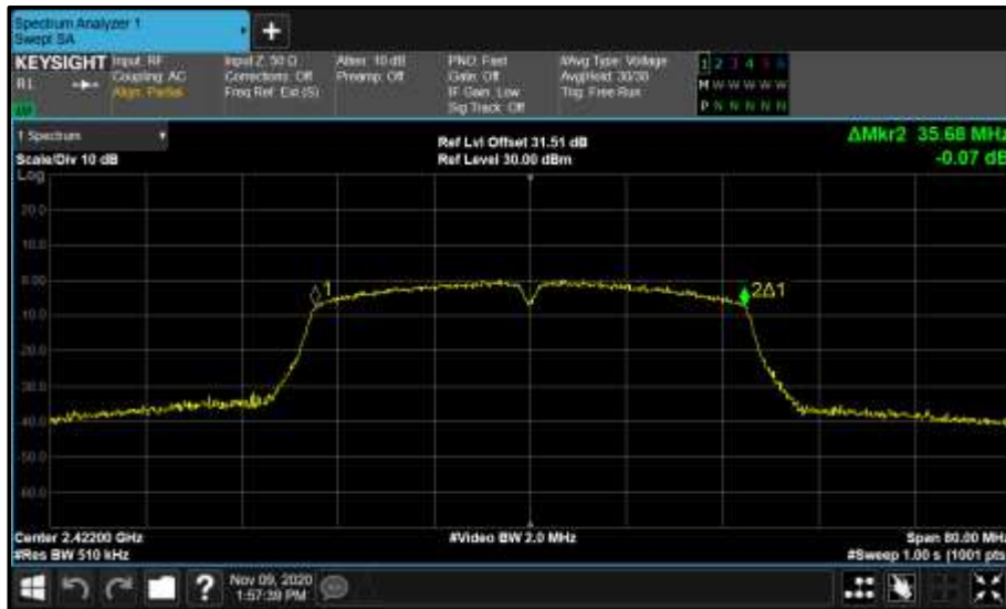
Figure 30 - Core 0 (A) 2422 MHz (CH3) 99% Bandwidth
