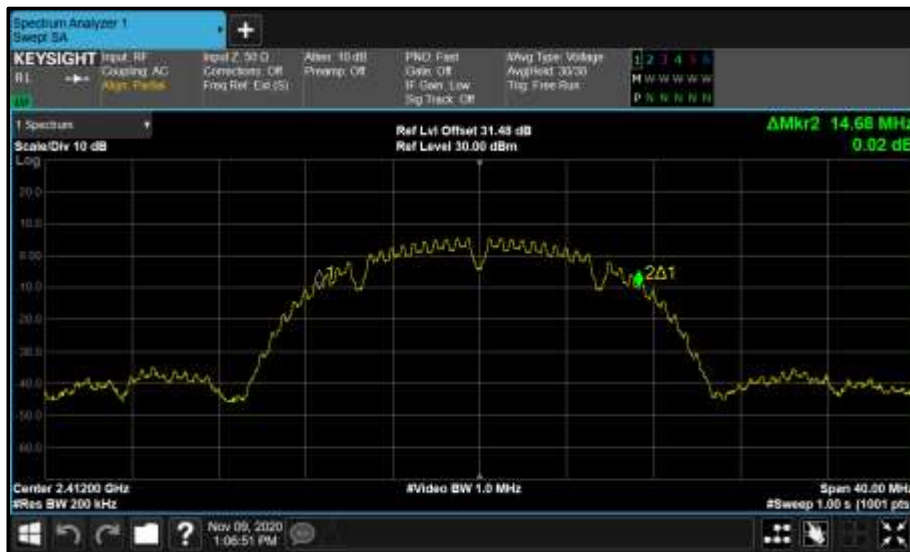
Figure 12 - Core 0 (A) 2412 MHz (CH1) 99% Bandwidth
