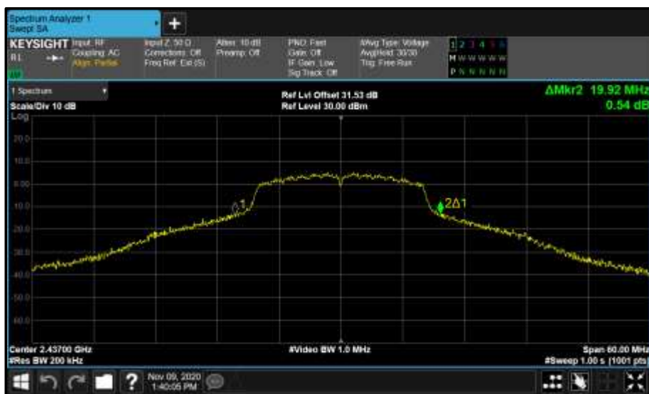
Figure 20 - Core 0 (A) 2437 MHz (CH6) 99% Bandwidth
