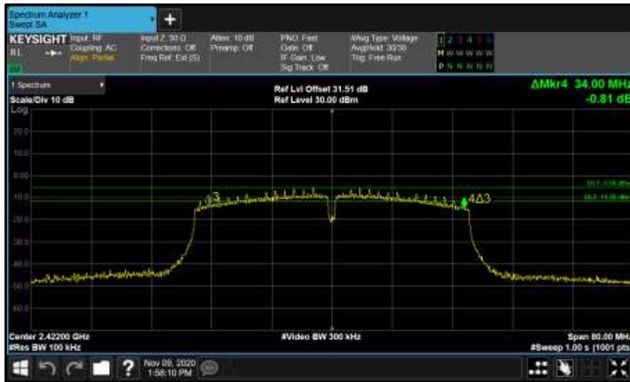
Figure 31 - Core 0 (A) 2422 MHz (CH3) 6 dB Bandwidth
