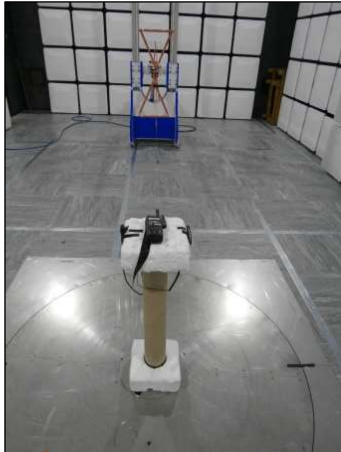
Figure 203 - Test Setup – 30 MHz to 1 GHz – X Orientation
