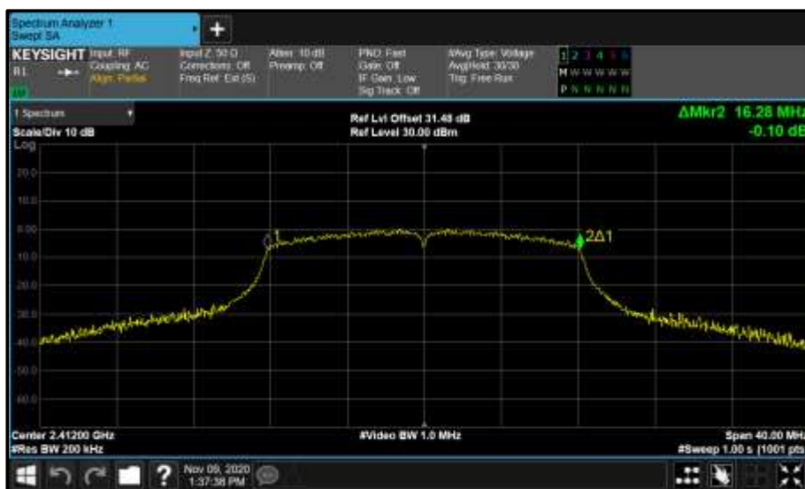
Figure 18 - Core 0 (A) 2412 MHz (CH1) 99% Bandwidth
