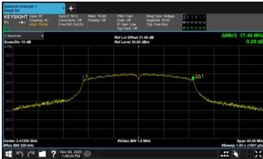
Figure 24 - Core 0 (A) 2412 MHz (CH1) 99% Bandwidth
