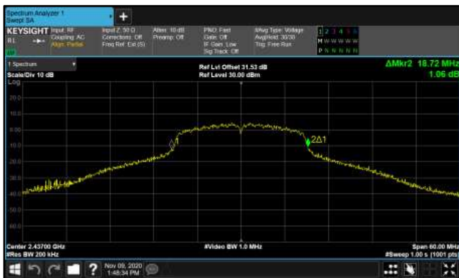
Figure 26 - Core 0 (A) 2437 MHz (CH6) 99% Bandwidth
