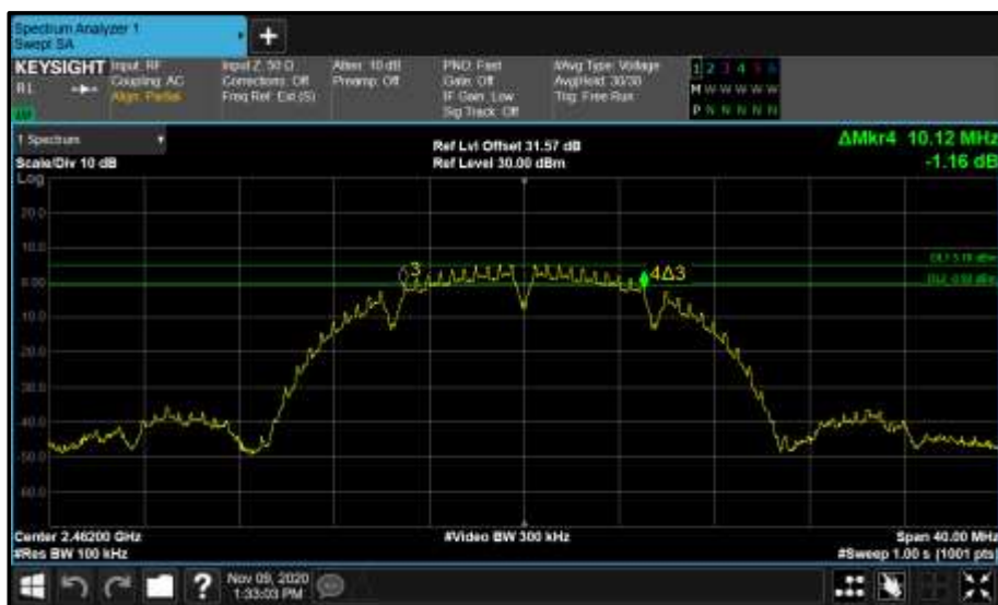
Figure 17 - Core 0 (A) 2462 MHz (CH11) 6 dB Bandwidth
