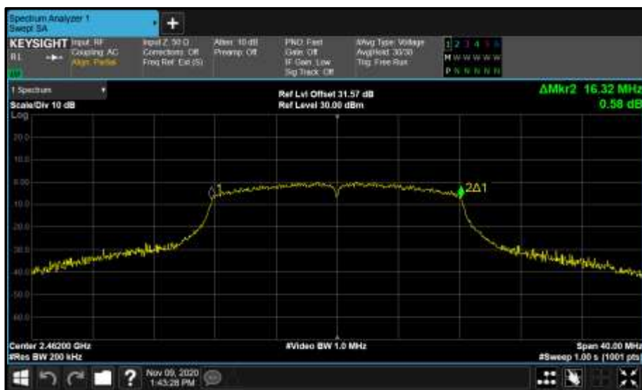
Figure 22 - Core 0 (A) 2462 MHz (CH11) 99% Bandwidth
