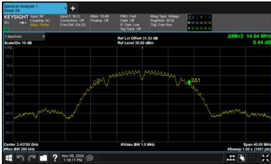
Figure 14 - Core 0 (A) 2437 MHz (CH6) 99% Bandwidth
