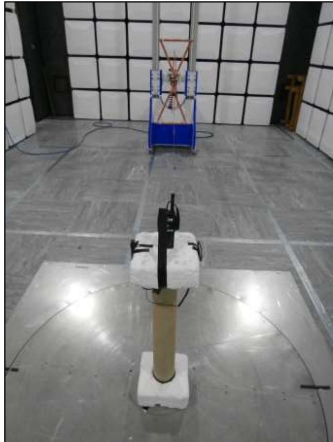
Figure 204 - Test Setup – 30 MHz to 1 GHz – Y Orientation
