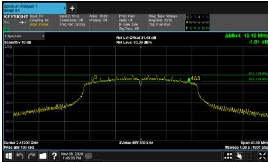
Figure 25 - Core 0 (A) 2412 MHz (CH1) 6 dB Bandwidth
