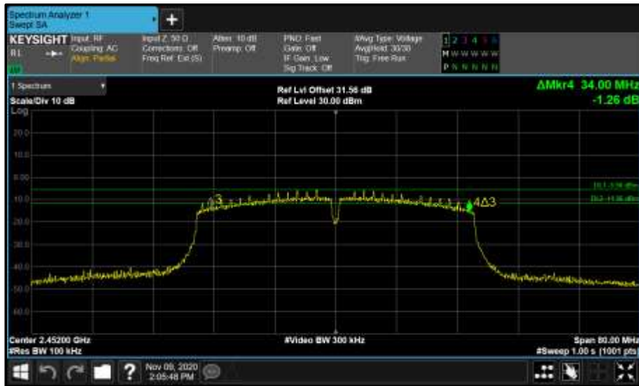
Figure 35 - Core 0 (A) 2452 MHz (CH9) 6 dB Bandwidth
