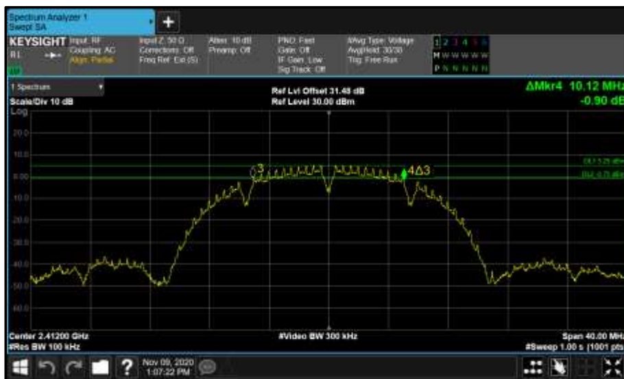
Figure 13 - Core 0 (A) 2412 MHz (CH1) 6 dB Bandwidth
