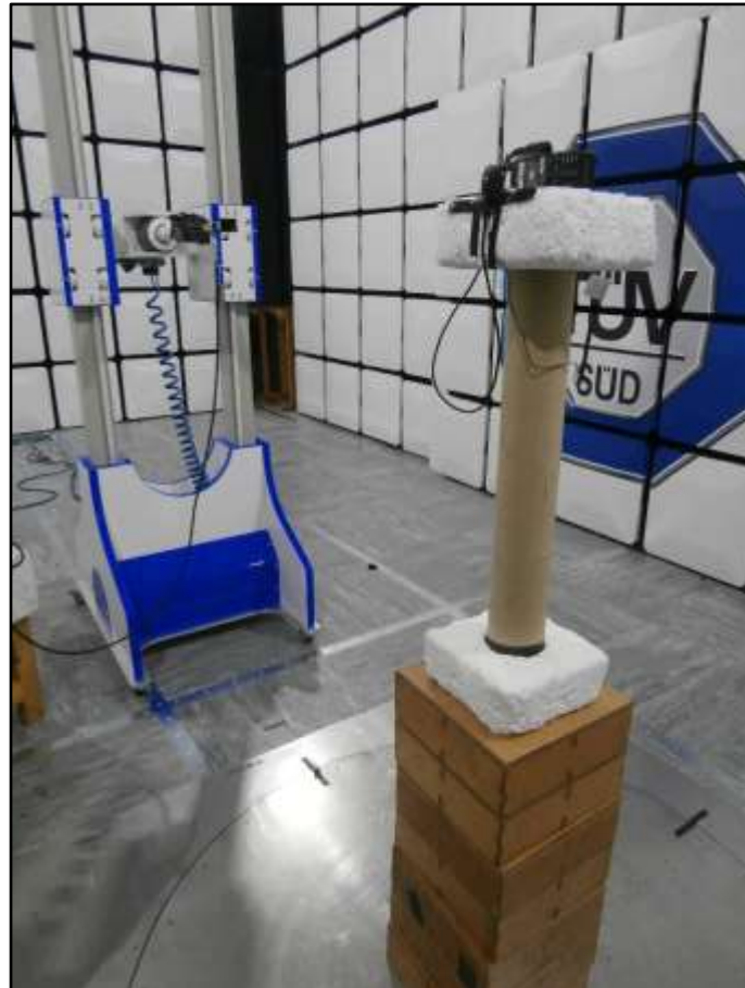
Figure 211 - Test Setup – 18 GHz to 25 GHz – Z Orientation
