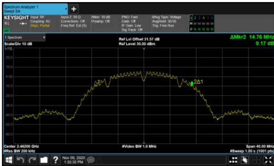
Figure 16 - Core 0 (A) 2462 MHz (CH11) 99% Bandwidth
