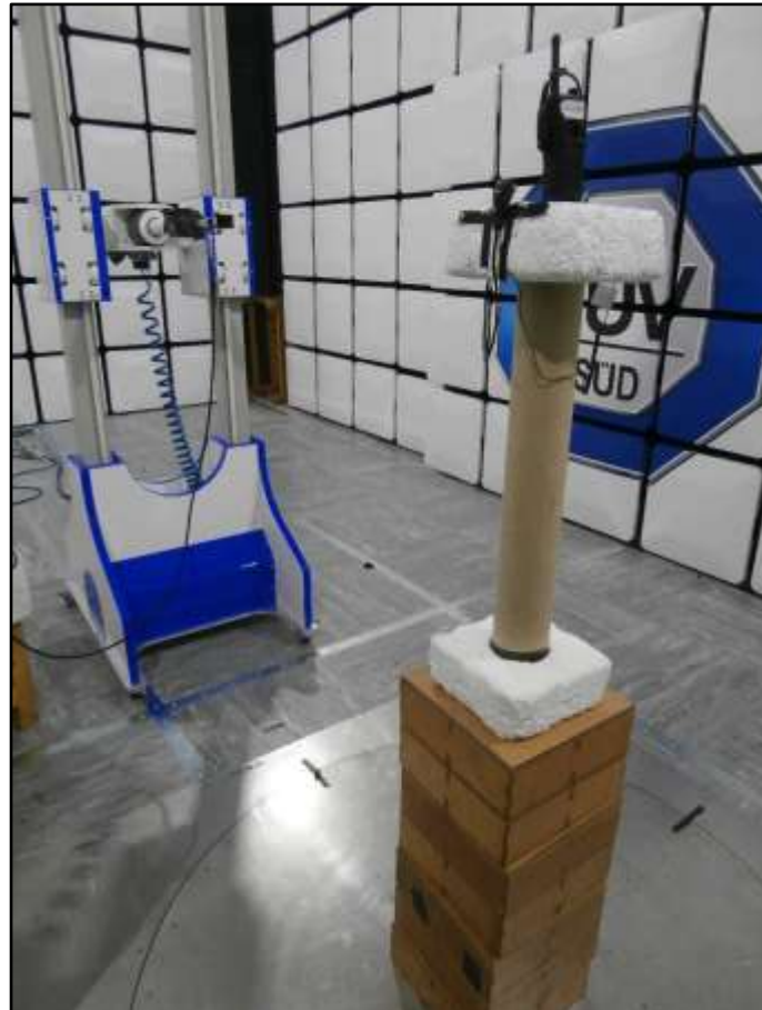
Figure 210 - Test Setup – 18 GHz to 25 GHz – Y Orientation
