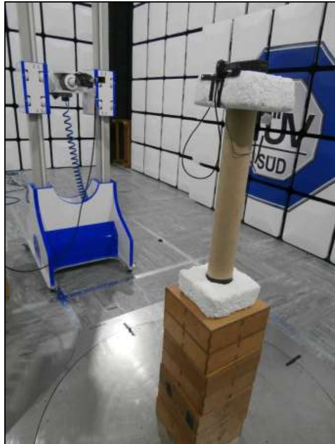
Figure 209 - Test Setup – 18 GHz to 25 GHz – X Orientation
