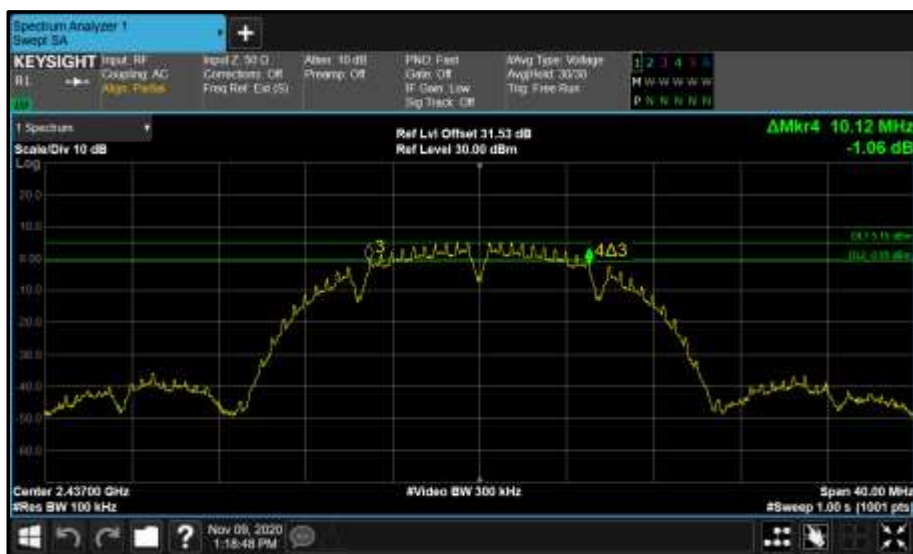
Figure 15 - Core 0 (A) 2437 MHz (CH6) 6 dB Bandwidth
