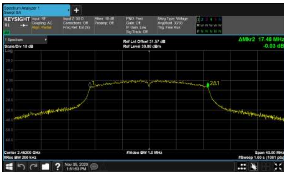
Figure 28 - Core 0 (A) 2462 MHz (CH11) 99% Bandwidth
