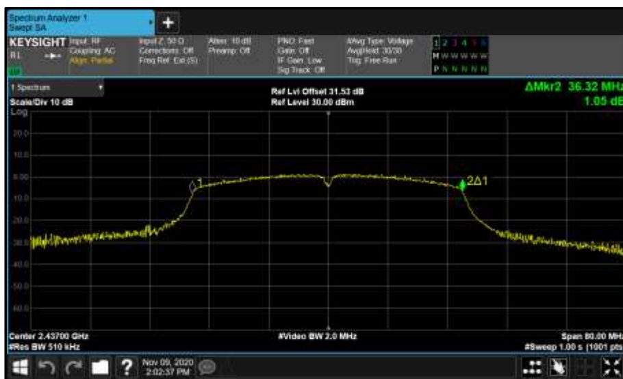
Figure 32 - Core 0 (A) 2437 MHz (CH6) 99% Bandwidth
