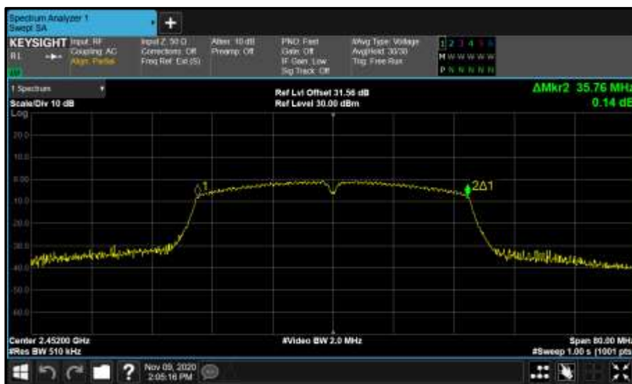
Figure 34 - Core 0 (A) 2452 MHz (CH9) 99% Bandwidth
