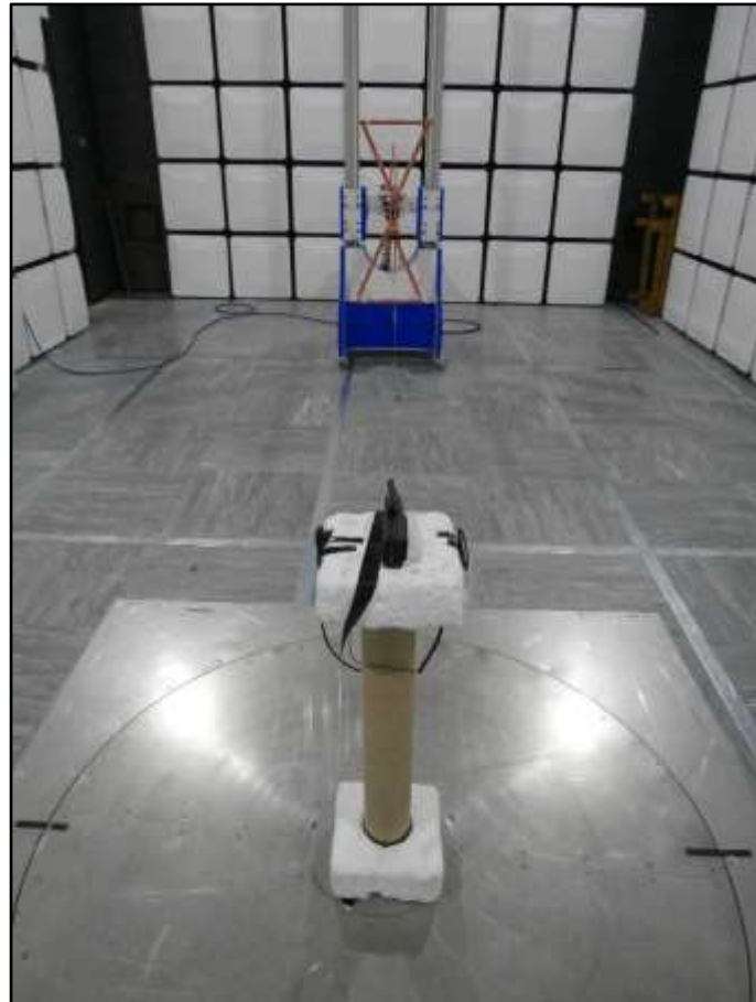
Figure 205 - Test Setup – 30 MHz to 1 GHz – Z Orientation
