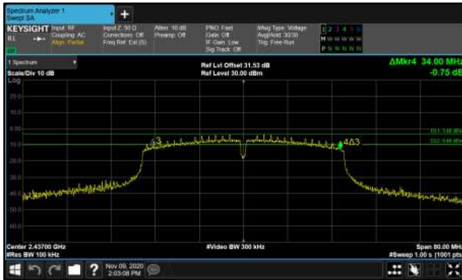
Figure 33 - Core 0 (A) 2437 MHz (CH6) 6 dB Bandwidth
