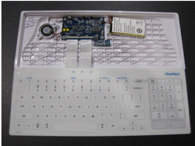
Figure 1 - CK3-15x keyboard containing CKW module and PPxMnnWx30 host.
