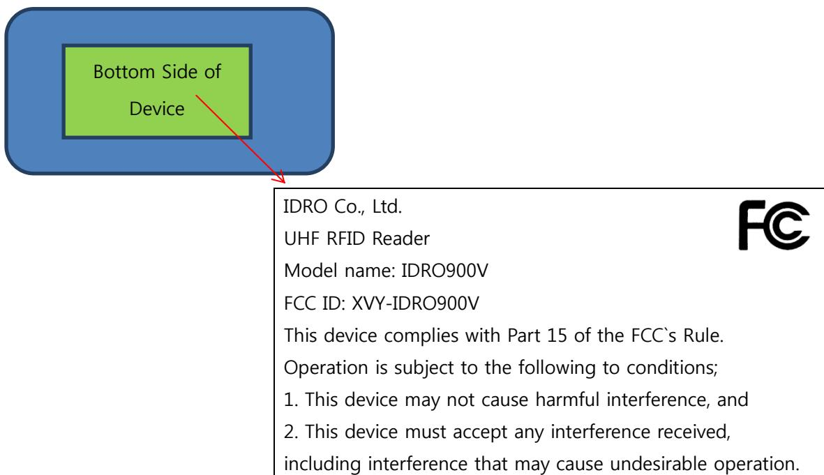
The label is attached to this device by an adhesive. The adhesive is permanent type with strong strength.
