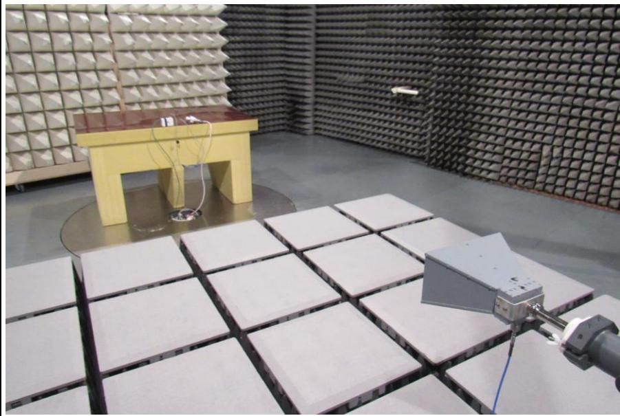
**TEST SETUP FOCUS RADIATED EMISSION**
