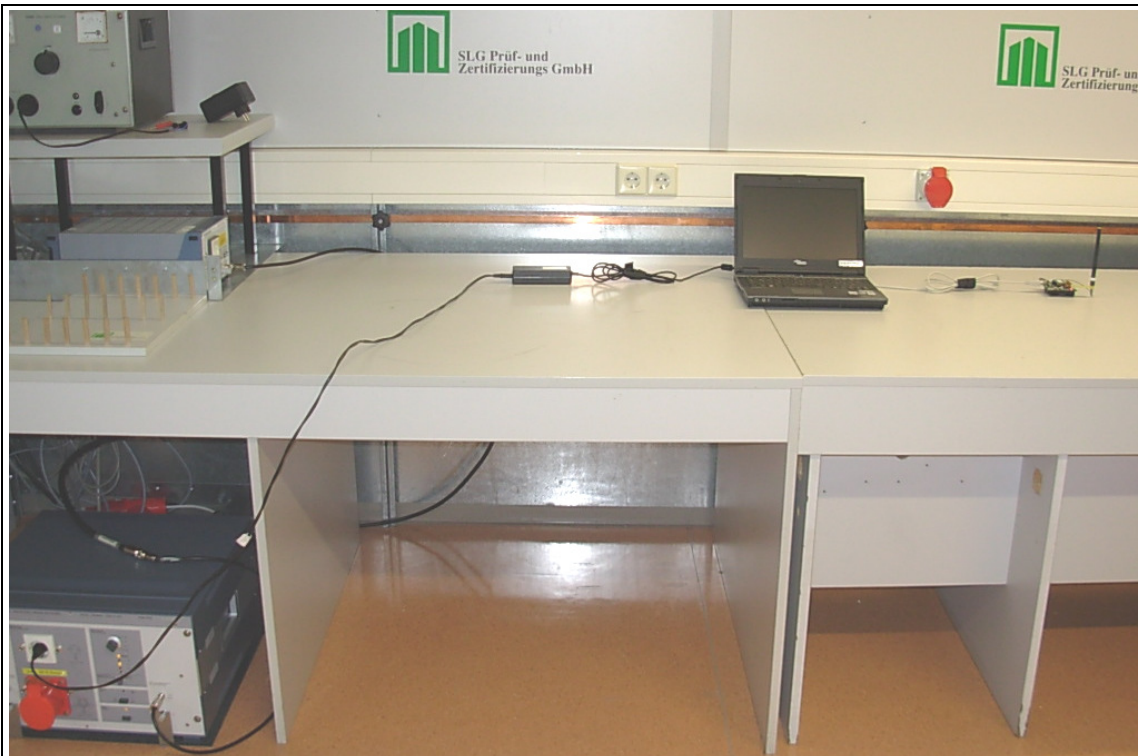
Figure 11: Measurement set-up for conducted measurement of disturbance voltage acc. to following section of the report 1114-11-EE-11-PB001: 4.6 and 4.7
