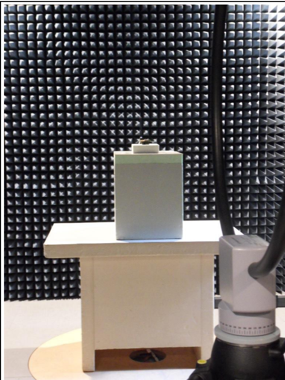
Figure 8: Measurement set-up for radiated measurement < 30 MHz acc. to following sections of the report 1114-11-EE-11-PB001: 4.4.1
