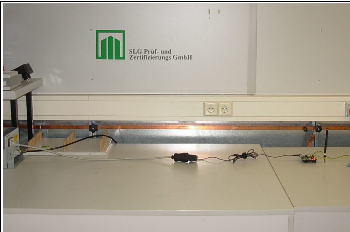
Figure 12: Measurement set-up for conducted measurement of disturbance voltage acc. to following section of the report 1114-11-EE-11-PB001: 4.6 and 4.7
