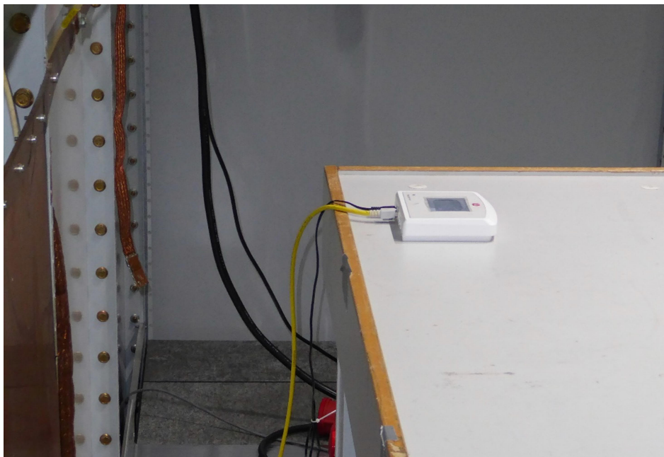
Test setup powerline conducted EUT with Ethernet connection (DC supplied, fping)
