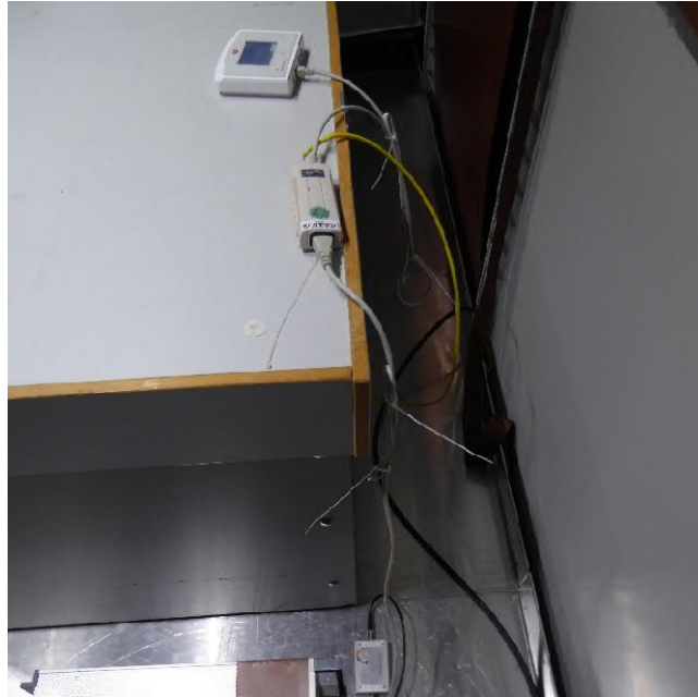
Test setup powerline conducted EUT with Ethernet connection (PoE supplied, fping)
