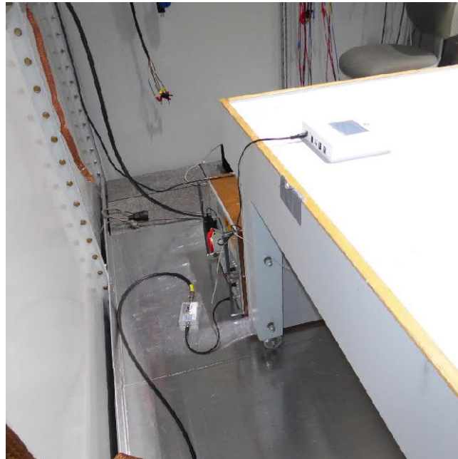
Test setup powerline conducted EUT in RX mode
