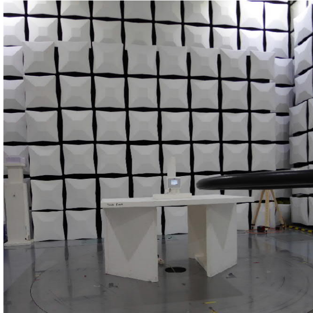
Antenna position 3 – grund-parallel Test setup semi-anechoic chamber M276
