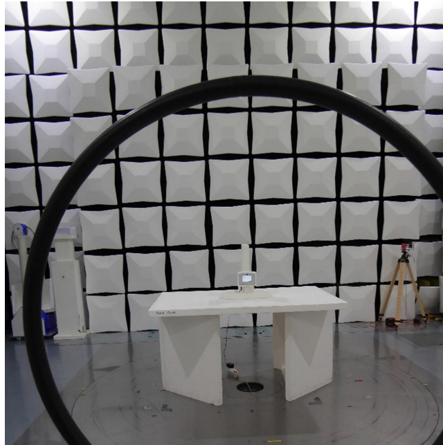
Antenna position 1 – parallel Test setup semi-anechoic chamber M276
