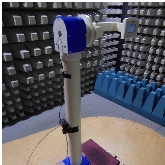
EUT on positioner Test setup fully anechoic chamber M20
