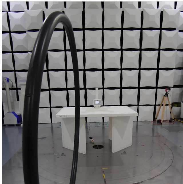
Antenna position 2 – perpendicular Test setup semi-anechoic chamber M276
