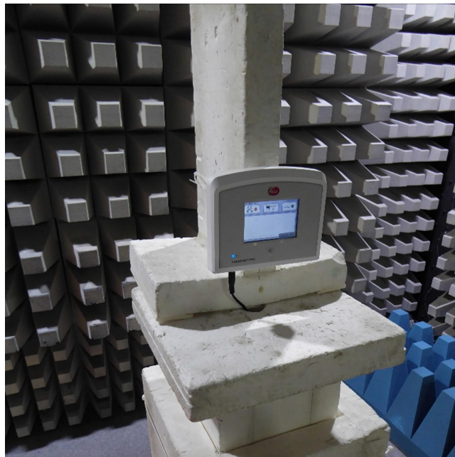
EUT position 1 Test setup fully anechoic chamber M20
