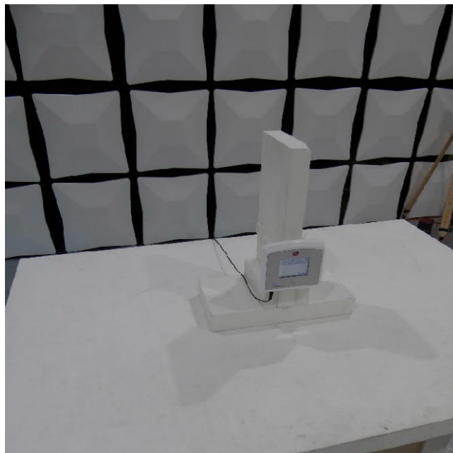
EUT Position Test setup semi-anechoic chamber M276
