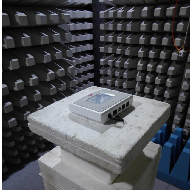
EUT position 2 Test setup fully anechoic chamber M20
