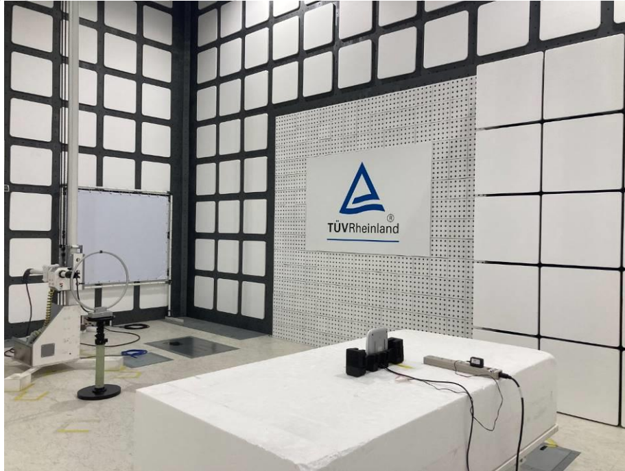
Photograph 4: Test Setup for Spurious Emissions (Back View 2)
