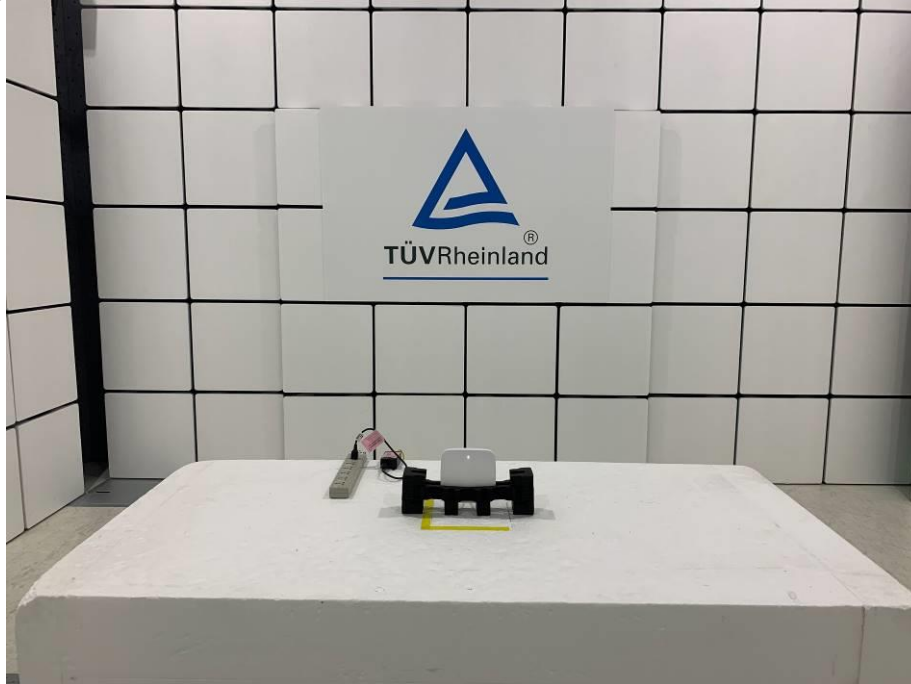
Photograph 9: Test Setup for Spurious Emissions (Front View 1)
