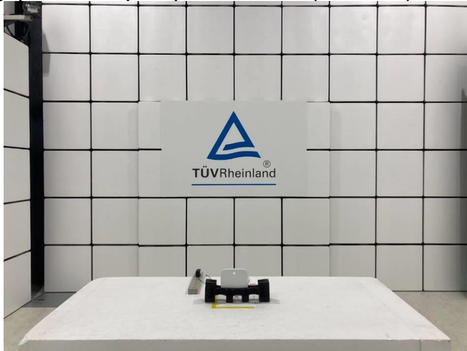
Photograph 2: Test Setup for Spurious Emissions (Front View 2)
