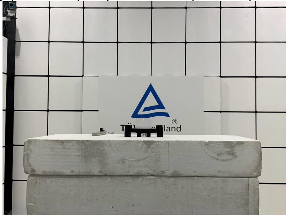
Photograph 2: Test Setup for Spurious Emissions (Front View 2)
