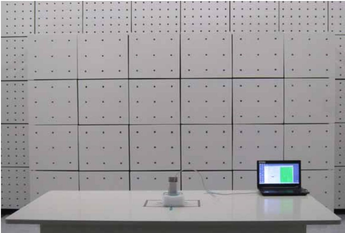
**Conducted Setup Photo (Measurement at Antenna Port)**
