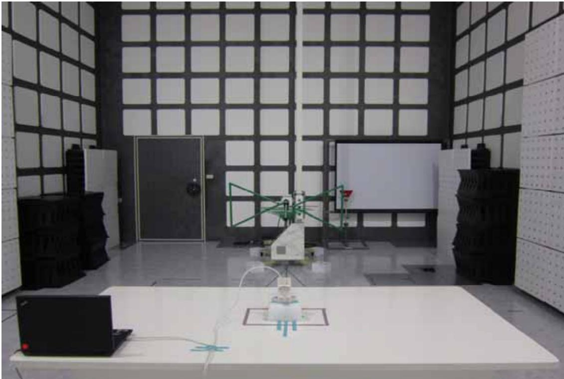
**Radiated Emission Set up Photos (E2 Plane) (Above 1G)**
