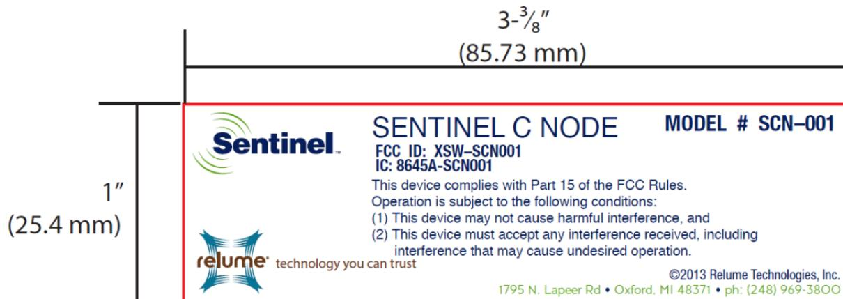
PLEASE APPLY LABEL TO OPPOSITE SIDE OF THE HOUSING FROM THE ALIGNMENT TAB. THIS IS USED DURING THE SONIC WELDING PROCESS
