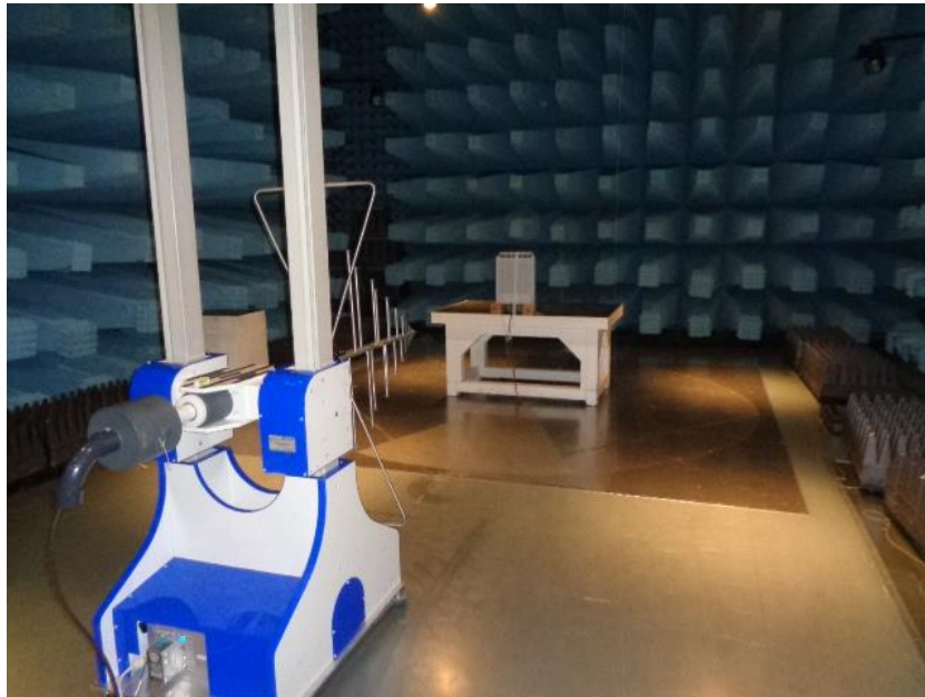
Figure 9.1-3: Radiated emissions set-up for frequencies below 1 GHz
