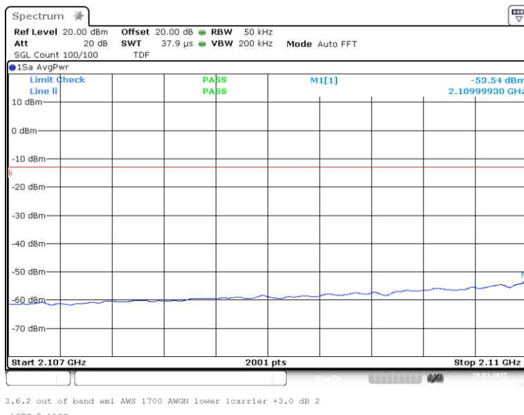
3.6.2 out of band emi AWS 1700 AWGN lower lcarrier +3.0 dB 2
