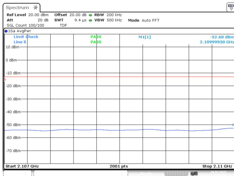
3.6.2 out of band emi AWS 1700 AWGN 45M lower lcarrier +3.0
