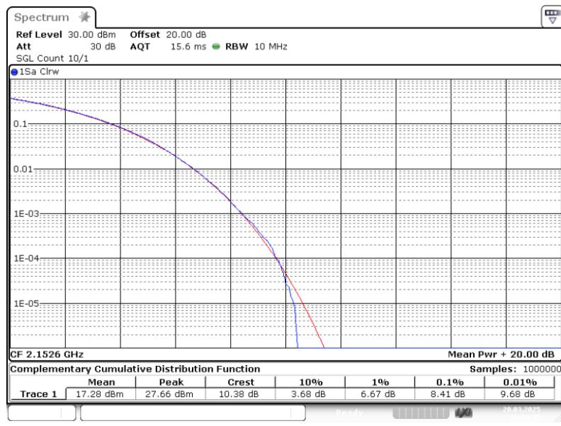
Band: AWS 1700; Frequency: 2.1526 GHz; Band edge: f0; Mod: AWGN; PAPR 3 dB > AGC
