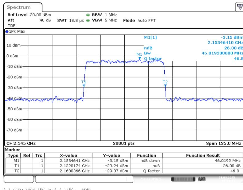
Band: AWS 1700; Frequency: 2.1450 GHz; Band edge: mid; Mod: AWGN 45M;
