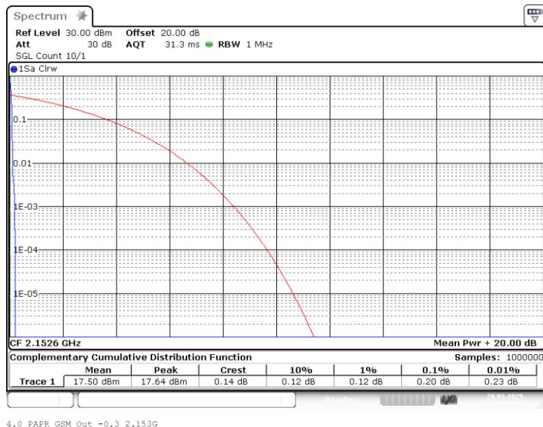
Band: AWS 1700; Frequency: 2.1526 GHz; Band edge: f0; Mod: GSM; PAPR 3 dB > AGC
