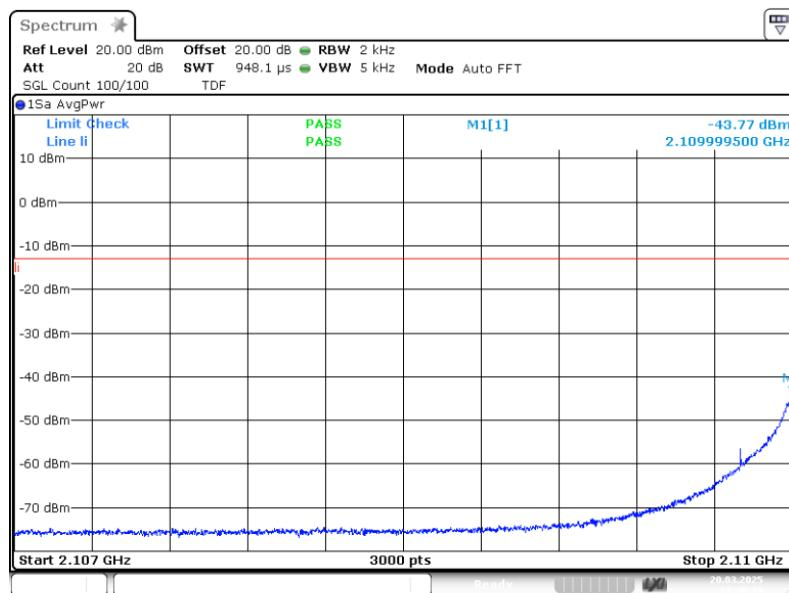
3.6.2 out of band emi AWS 1700 GSM lower 2carriers +3.0 dB 2
