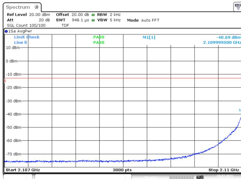
3.6.2 out of band emi AWS 1700 GSM lower lcarrier -0.3 dB 2.
