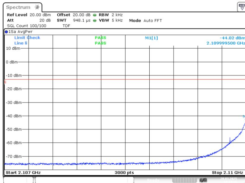
3.6.2 out of band emi AWS 1700 GSM lower 2carriers -0.3 dB 2
