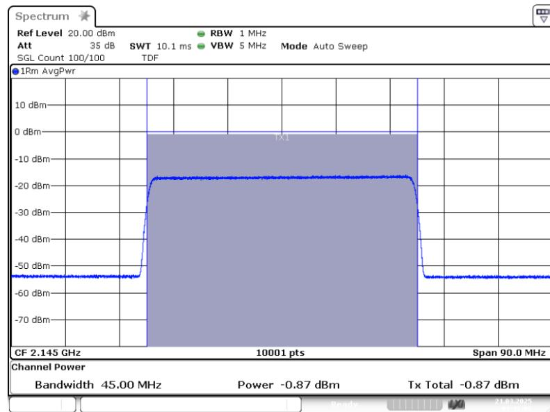
Band: AWS 1700; Frequency: 2.1450 GHz; Band edge: mid; Mod: AWGN 45M;
