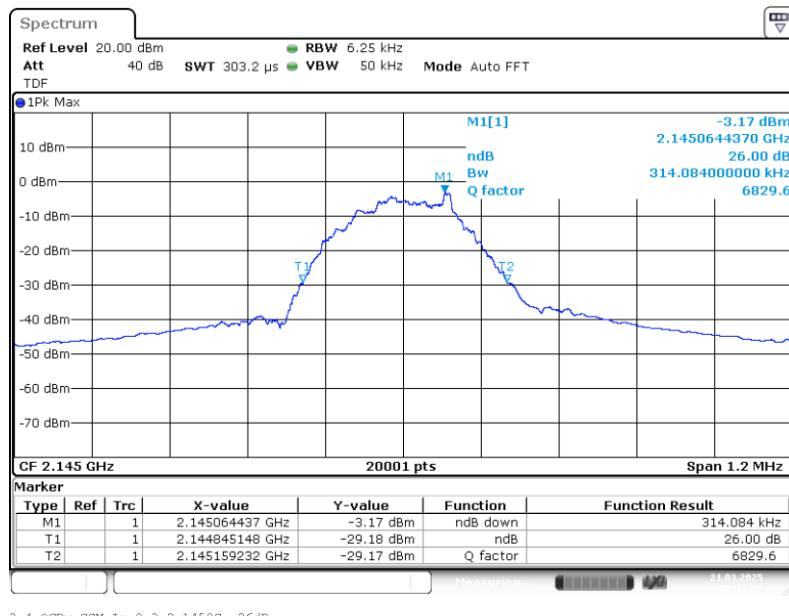
Band: AWS 1700; Frequency: 2.1450 GHz; Band edge: mid; Mod: GSM;
