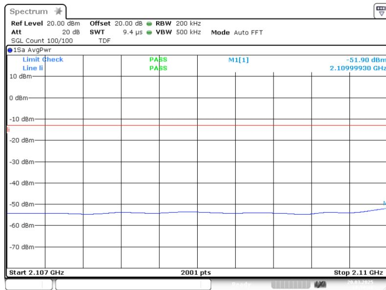
3.6.2 out of band emi AWS 1700 AWGN 45M lower lcarrier -0.3
