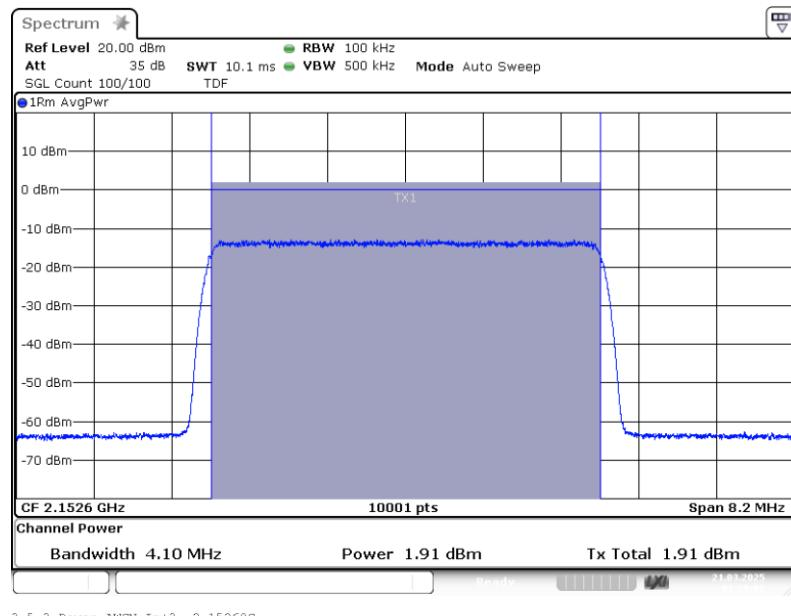
Band: AWS 1700; Frequency: 2.1526 GHz; Band edge: f0; Mod: AWGN;
