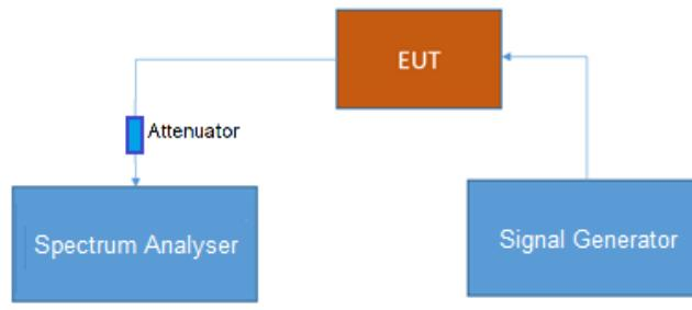
Test Setup step 2; Occupied Bandwidth/Input-versus-output spectrum
