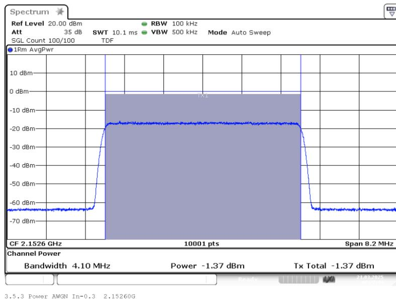
Band: AWS 1700; Frequency: 2.1526 GHz; Band edge: f0; Mod: AWGN;
