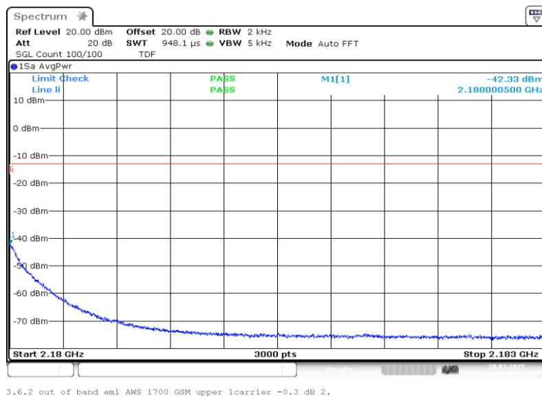
Band: AWS 1700; Frequency: 2.1100 GHz to 2.1800 GHz; Band edge: upper; Mod: GSM;
