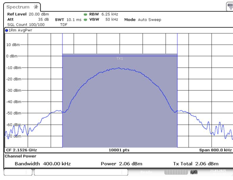
Band: AWS 1700; Frequency: 2.1526 GHz; Band edge: f0; Mod: GSM;
