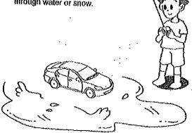
5. Point your transmitter antenna up not down toward your vehicle.If your vehicle gets too far away, it won't work properly. If your transmitter have an antenna carry-loop feature, make sure the antenna is remove from the holder and straighening before operating.
