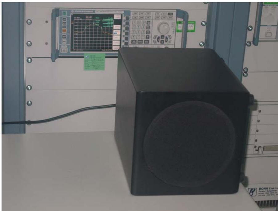
Set-up for Power Spectral Density and 99% Bandwidth test
