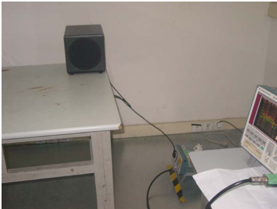
Set-up for conducted emission at the mains terminals test
