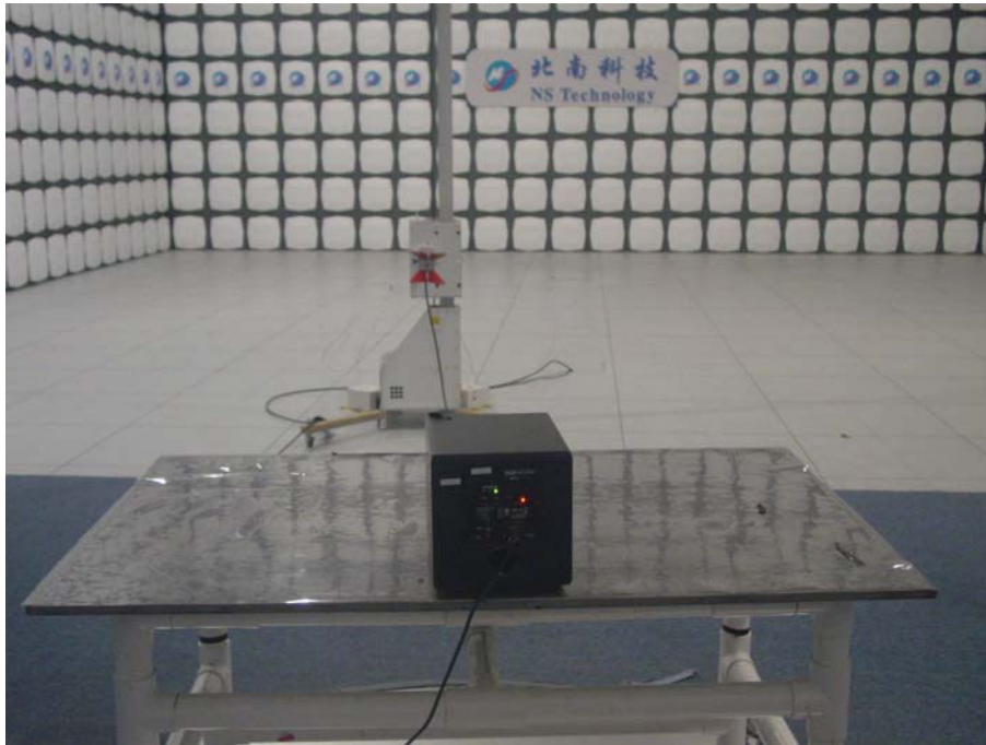
Set-up for radiated emission test (Above 1GHz)
