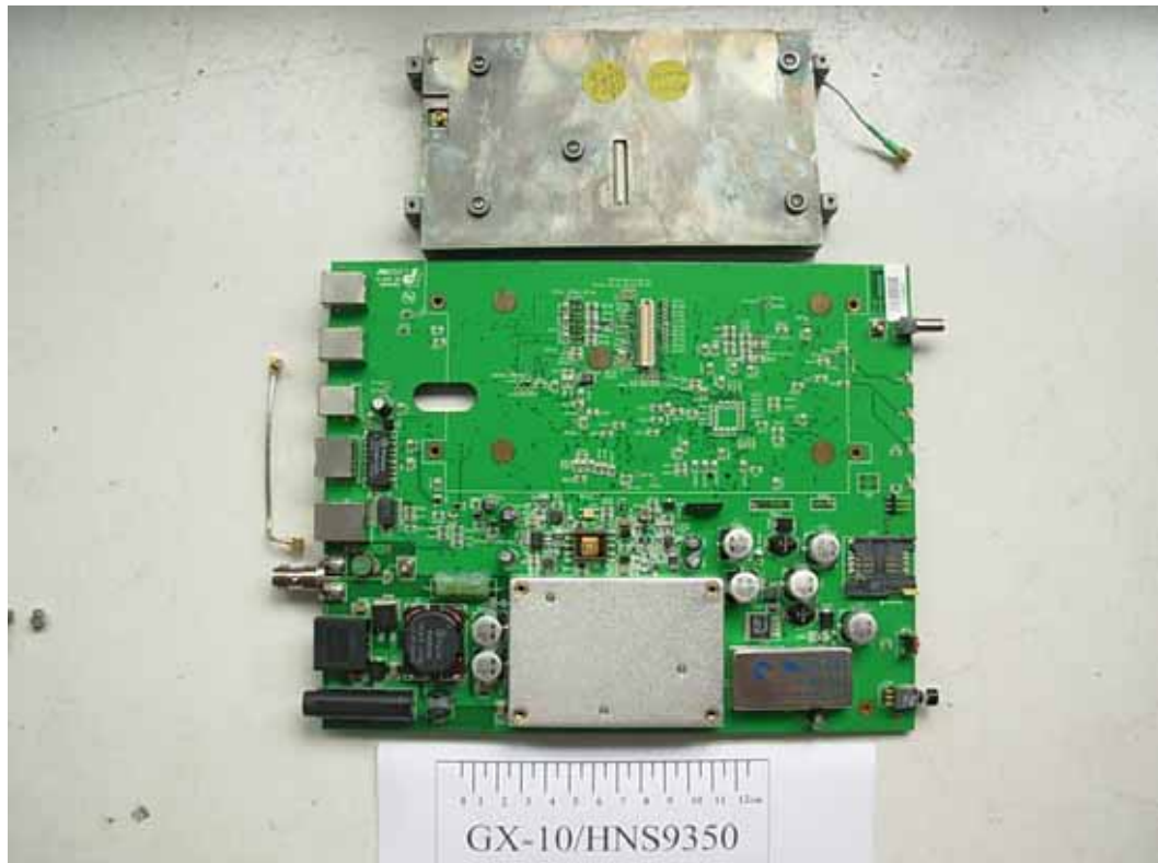
FIGURE 11 INMARSAT BGAN LVUT (M/N: GX-10) MAIN BOARD – MODULE REMOVED
