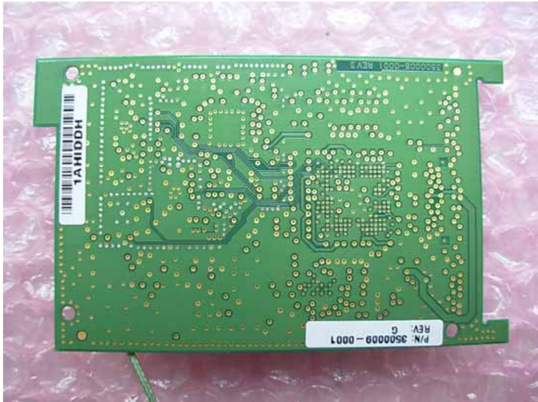
FIGURE 19 INMARSAT BGAN LVUT (M/N: GX-10) MAIN BOARD - MODULE – BOARD SIDE 2
