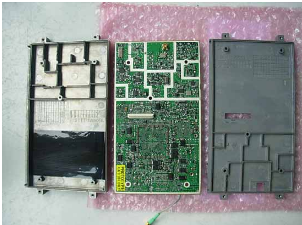
FIGURE 12 INMARSAT BGAN LVUT (M/N: GX-10) MAIN BOARD - MODULE – COVER REMOVED
