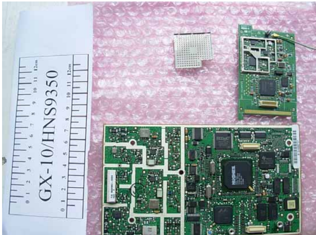
FIGURE 13 INMARSAT BGAN LVUT (M/N: GX-10) MAIN BOARD - MODULE – BOARD REMOVED
