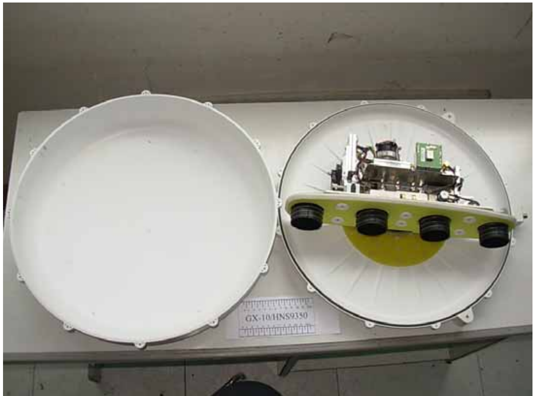
FIGURE 22 INMARSAT BGAN LVUT (M/N: GX-10) SATELLITE ANTENNA – COVER REMOVED
