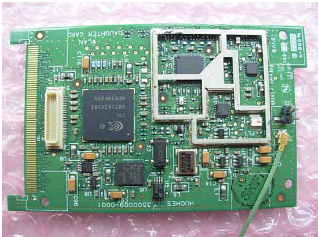
FIGURE 18 INMARSAT BGAN LVUT (M/N: GX-10) MAIN BOARD - MODULE – BOARD SIDE 1
