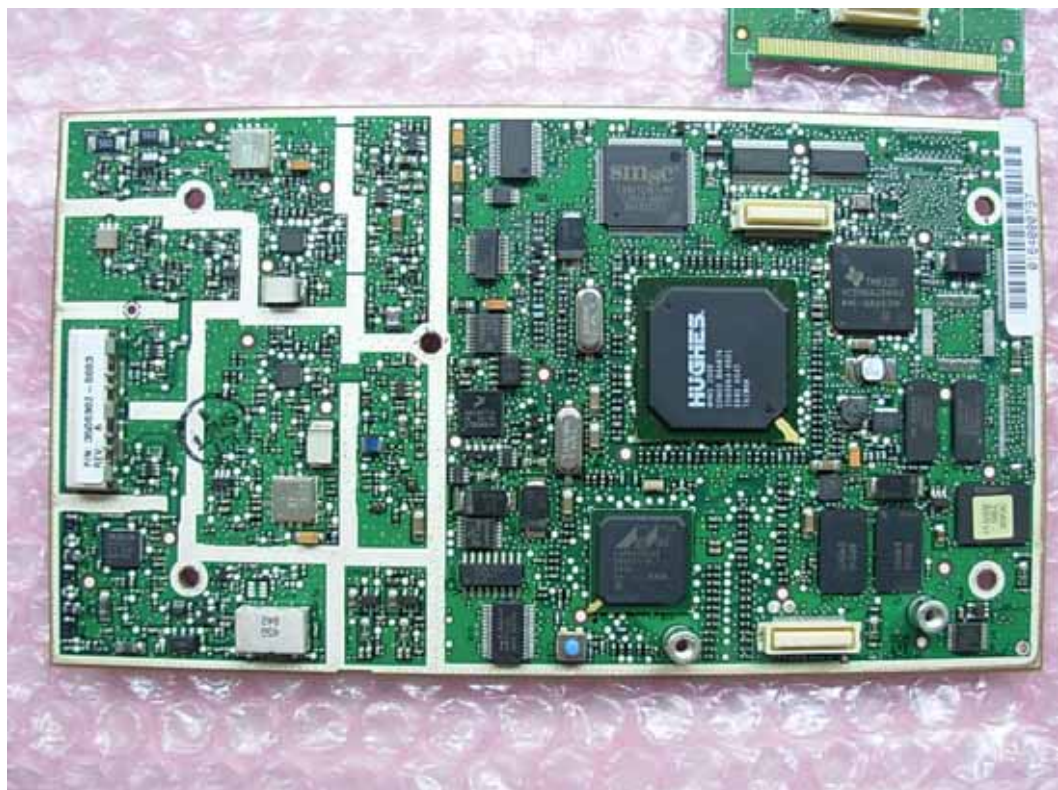
FIGURE 14 INMARSAT BGAN LVUT (M/N: GX-10) MAIN BOARD - MODULE – SIDE 1
