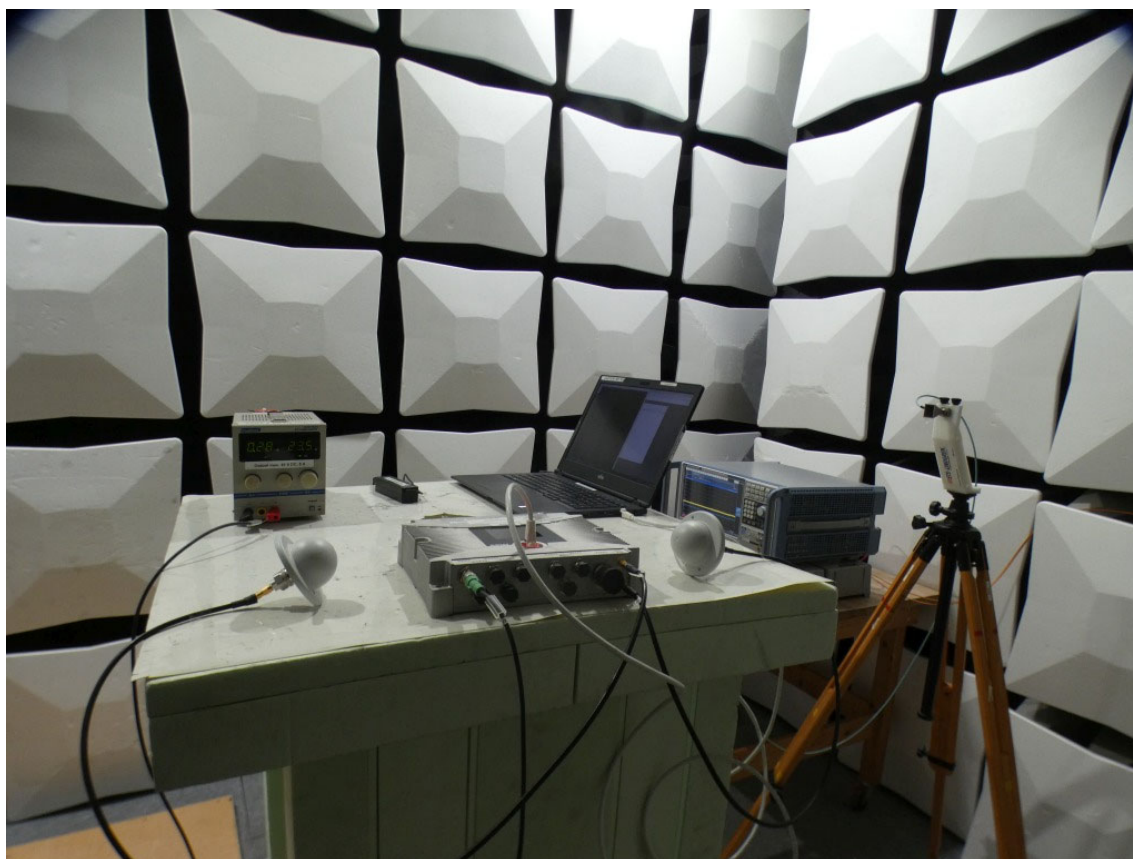
Photo 3: Test setup for radiated measurements (semi-anechoic chamber + mobile floor absorber, computer peripheral Setup for 26 GHz – 40 GHz ; unintentional radiator §15.109, ANSI C63.4)
