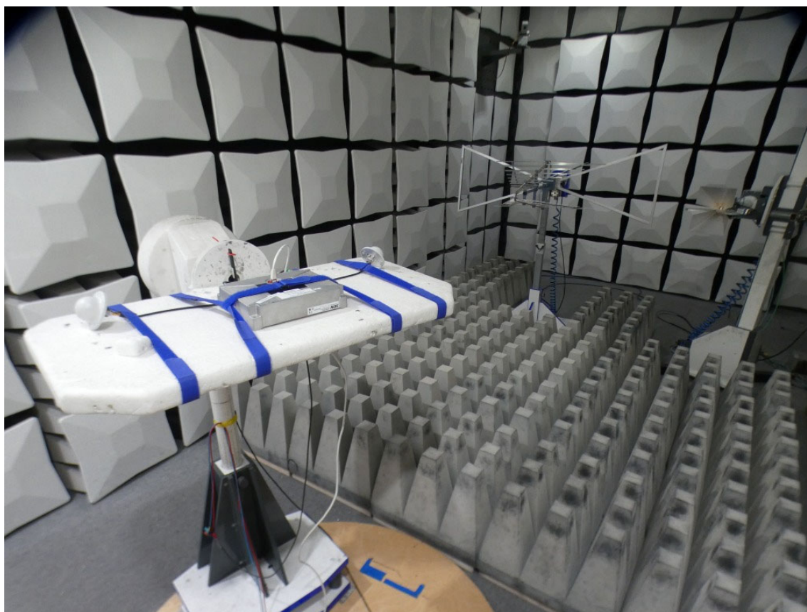
Photo 5: Test setup for radiated measurements (fully-anechoic chamber, Standalone Setup for 1 GHz – 24 GHz)
