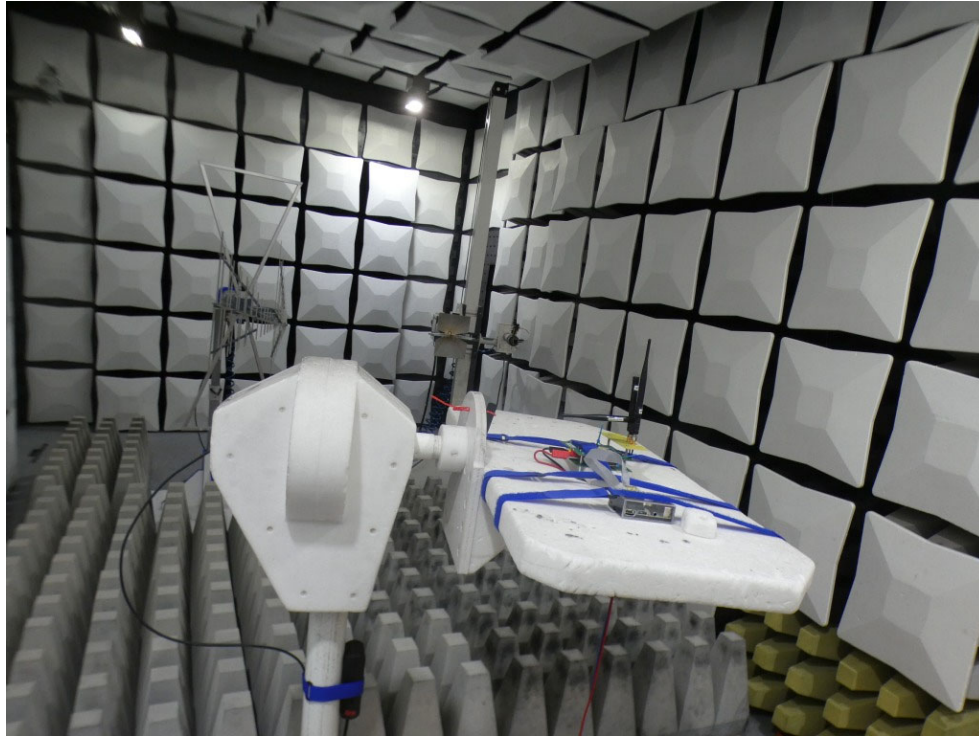
Photo 5: Test setup for radiated measurements above 1 GHz
