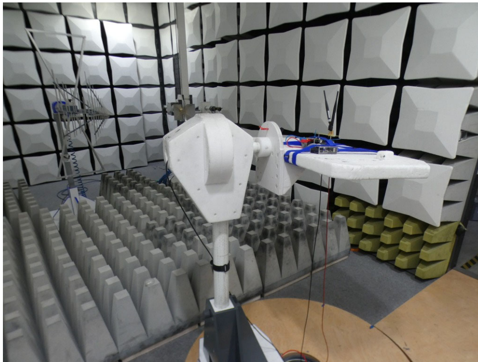
Photo 6: Test setup for radiated measurements above 1 GHz
