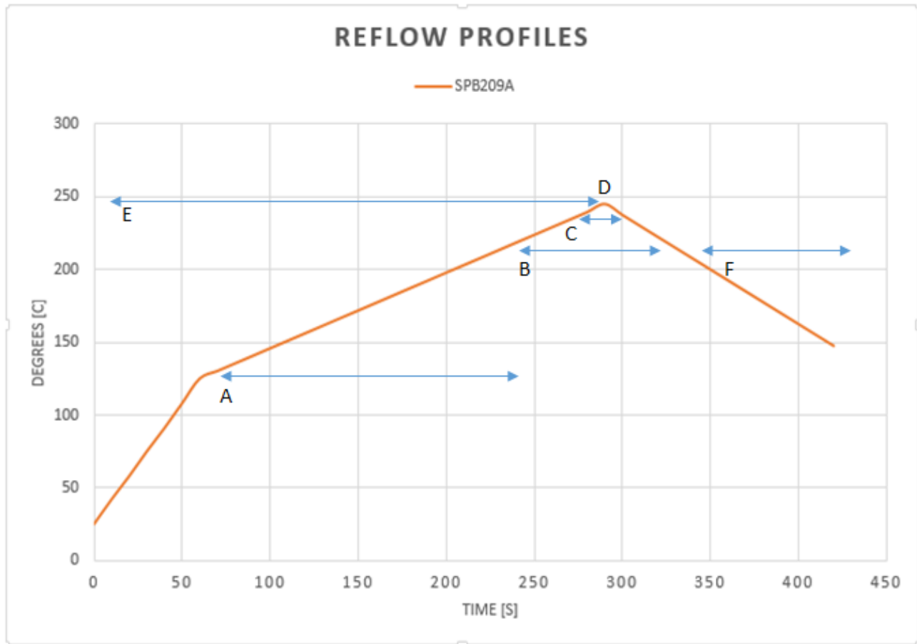
Figure 5-1: Reflow Temperature Profile
