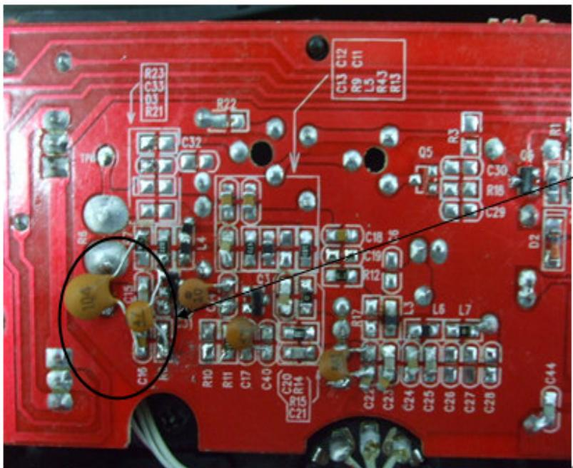
Add  $C_{16}=0.1\mu F$  capacitance and  $C_a=47pF$  capacitance to these positions; after modify:
