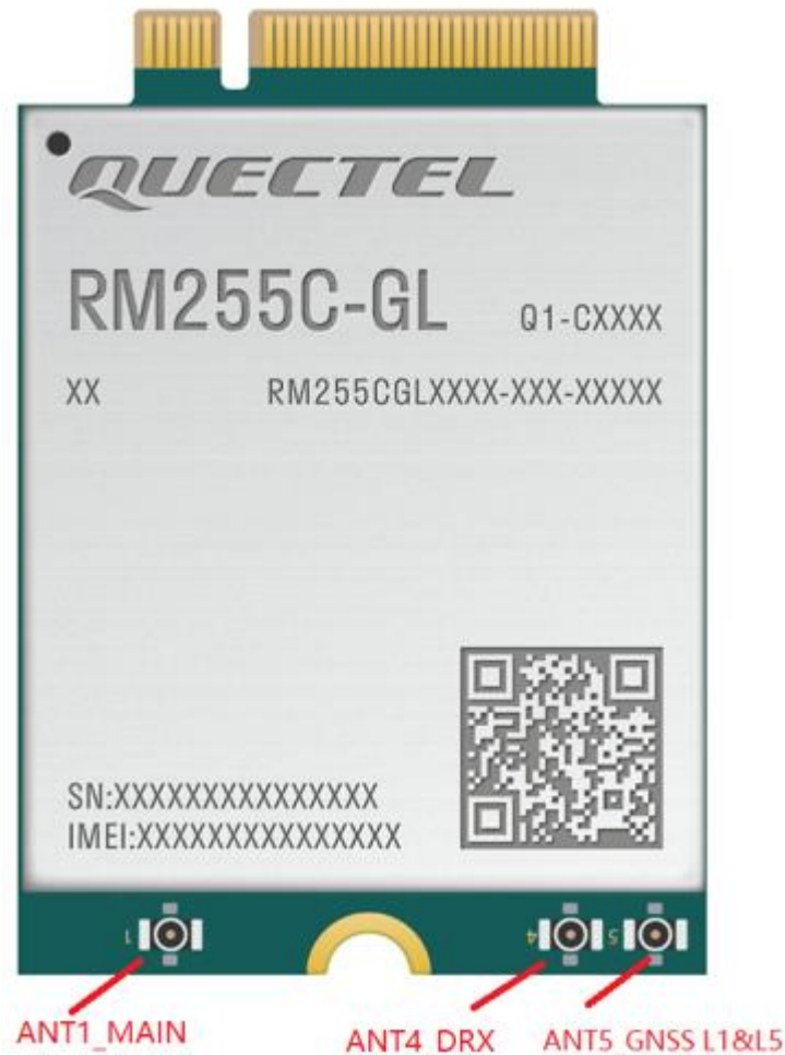
Figure 29: RM255C-GL Antenna Connectors
