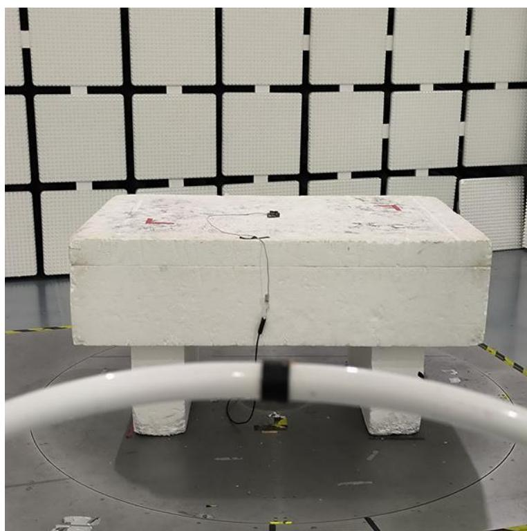
**Radiated Emissions Test Photos****30 MHz to 1000 MHz**
