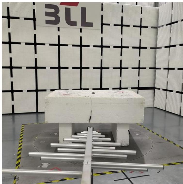
**Radiated Emissions Test Photos****Above 1 GHz**
