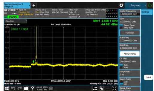
NTNV-n78(3700-3800)-PC2-30-50-L-DFT-BPSK-Inner_1RB_Right-300 0-6000-PASS
