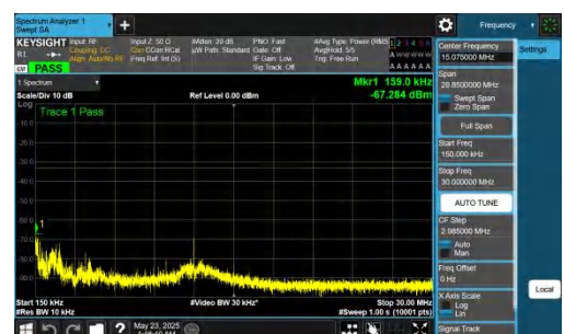
NTNV-n78(3700-3800)-PC2-30-25-M-DFT-QPSK-Inner_1RB_Left-0.15-30-PASS
