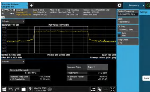
NTNV-n78(3700-3800)-PC2-30-90-M-CP-64QAM-Outer_Full-Ant1-PA
