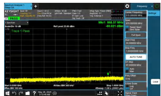
NTNV-n77(3450-3550)-PC2-30-60-H-DFT-QPSK-Inner_1RB_Right-30-1000-PASS
