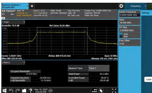
NTNV-n77(3450-3550)-PC2-30-15-M-CP-64QAM-Outer_Full-Ant1-PA
