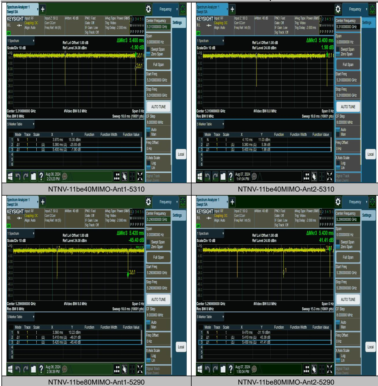
**Maximum conducted output power****Test Result**
