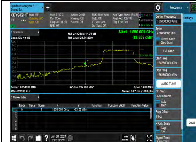
QPSK High channel-1 RB offset max
