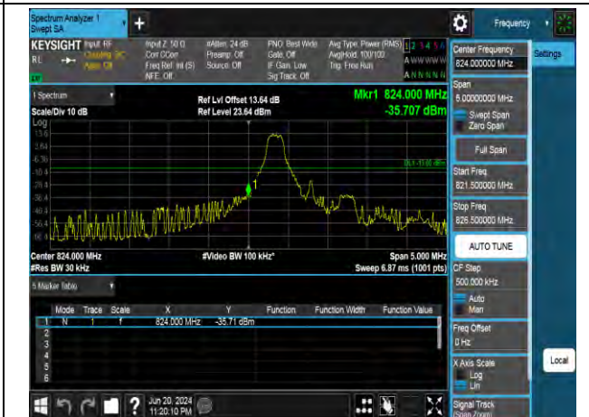
16QAM Low channel-1 RB offset 0
