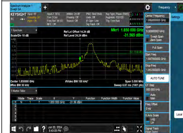
QPSK Low channel-6 RB offset 0
