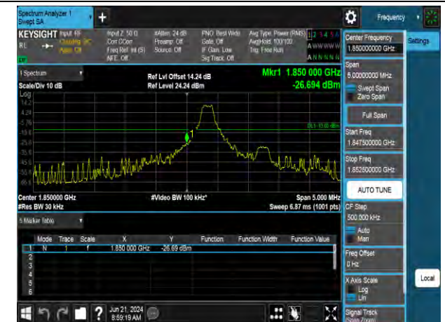
16QAM Low channel-1 RB offset 0
