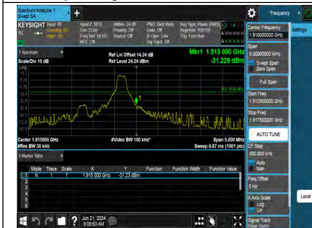
QPSK High channel-6 RB offset 0
