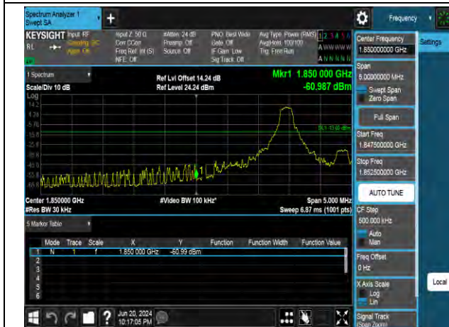
QPSK Low channel-1 RB offset 0
