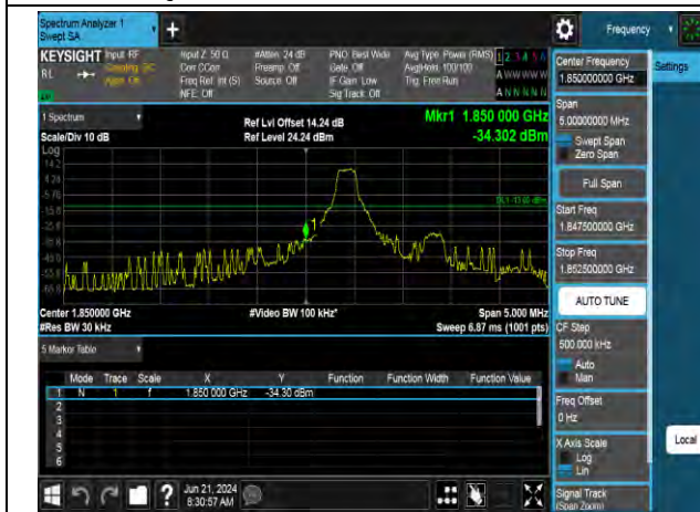
QPSK Low channel-6 RB offset 0
