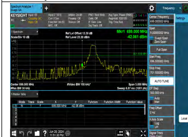
QPSK Low channel-1 RB offset 0
