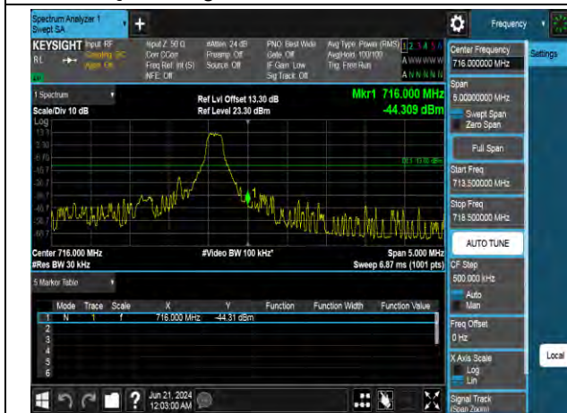
QPSK High channel-6 RB offset 0
