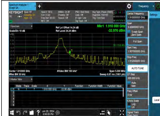
QPSK High channel-6 RB offset 0
