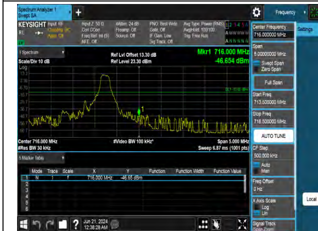
QPSK High channel-6 RB offset 0
