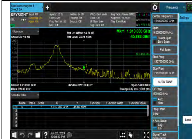
QPSK High channel-6 RB offset 0
