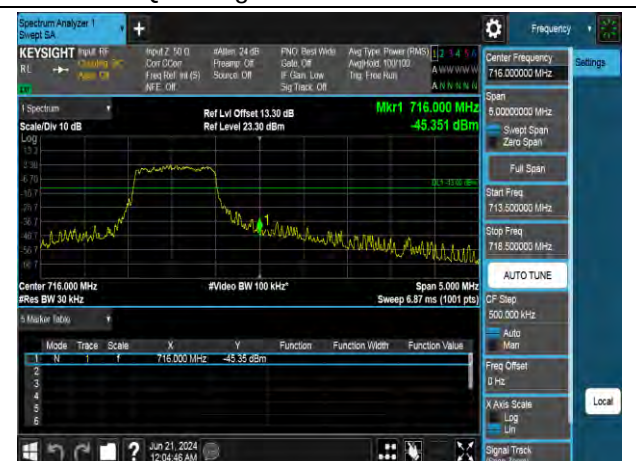
16QAM High channel-5 RB offset 0
