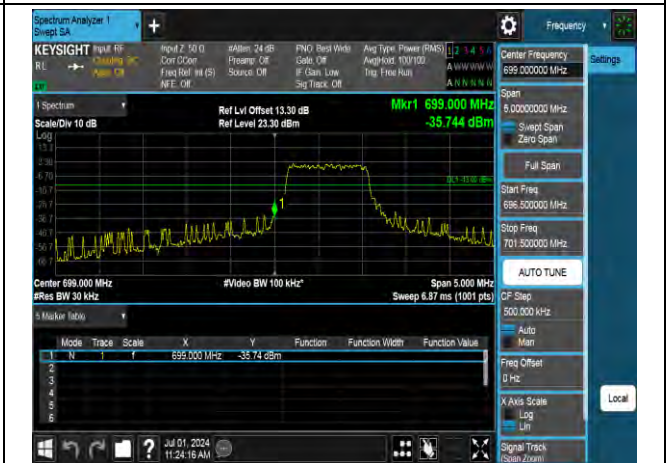
16QAM Low channel-5 RB offset 0
