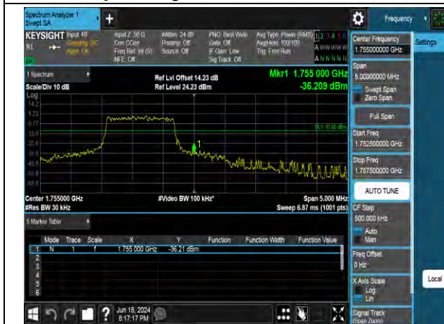
QPSK High channel-6 RB offset 0
