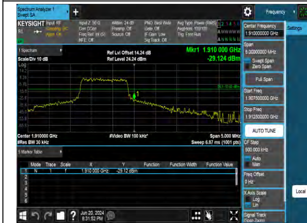
QPSK High channel-6 RB offset 0
