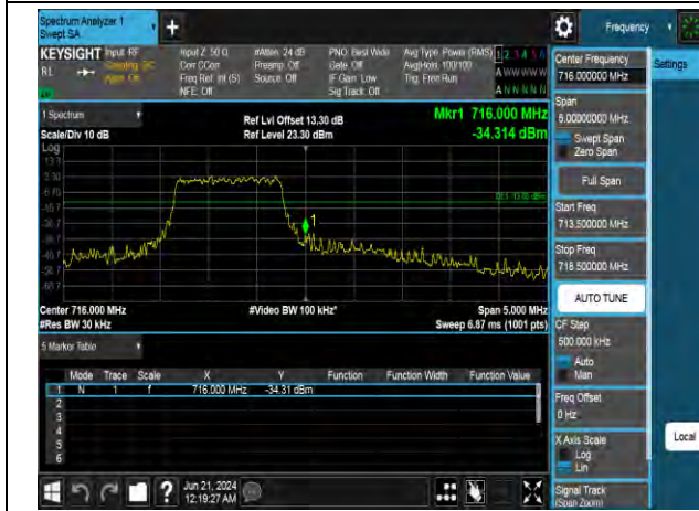
QPSK High channel-6 RB offset 0
