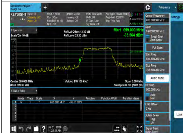
QPSK Low channel-6 RB offset 0
