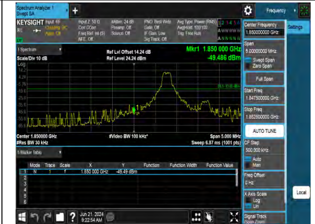
16QAM Low channel-5 RB offset 0
