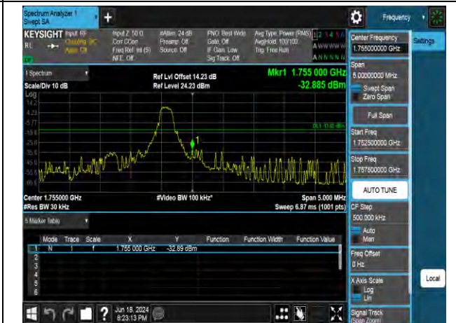
16QAM High channel-5 RB offset 0
