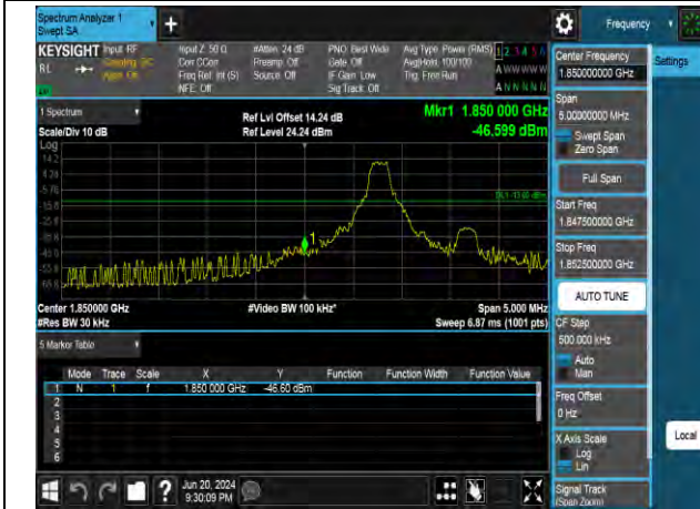
QPSK Low channel-6 RB offset 0
