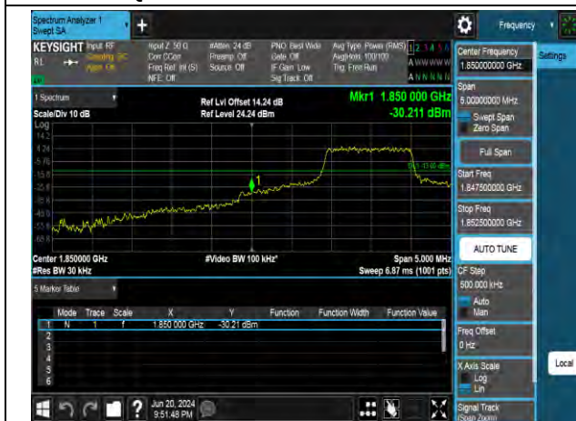
QPSK Low channel-6 RB offset 0
