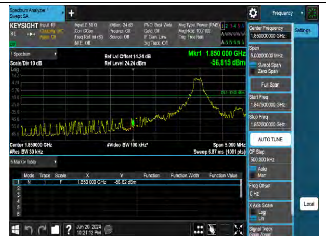
16QAM Low channel-1 RB offset 0
