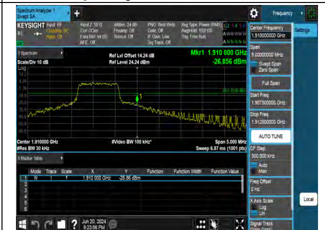
16QAM High channel-5 RB offset 0
