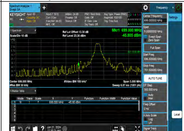
16QAM Low channel-1 RB offset 0
