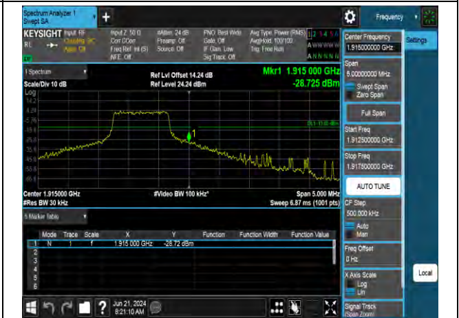
16QAM High channel-5 RB offset 0
