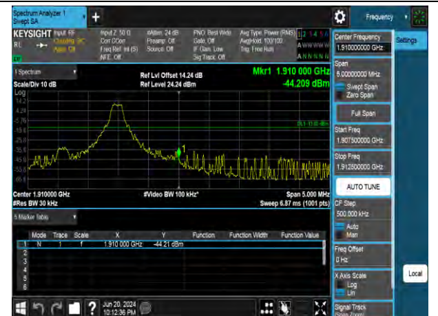
16QAM High channel-5 RB offset 0
