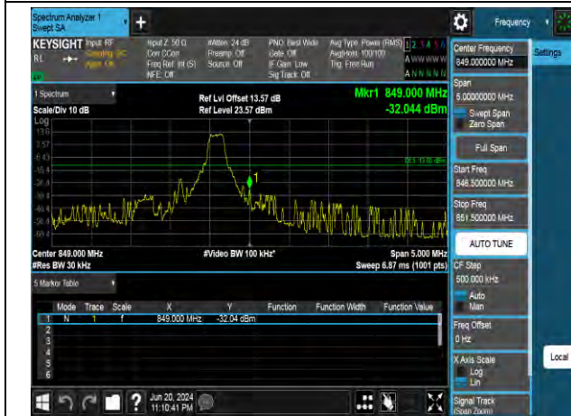
QPSK High channel-6 RB offset 0
