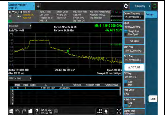
16QAM High channel-5 RB offset 0
