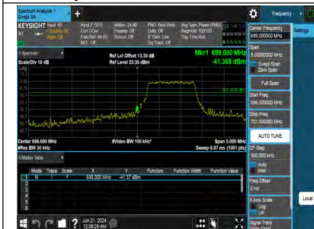
QPSK High channel-1 RB offset max
