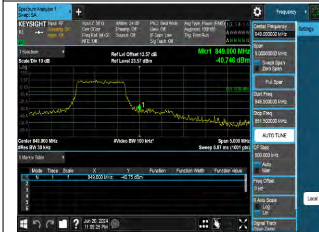
QPSK High channel-6 RB offset 0
