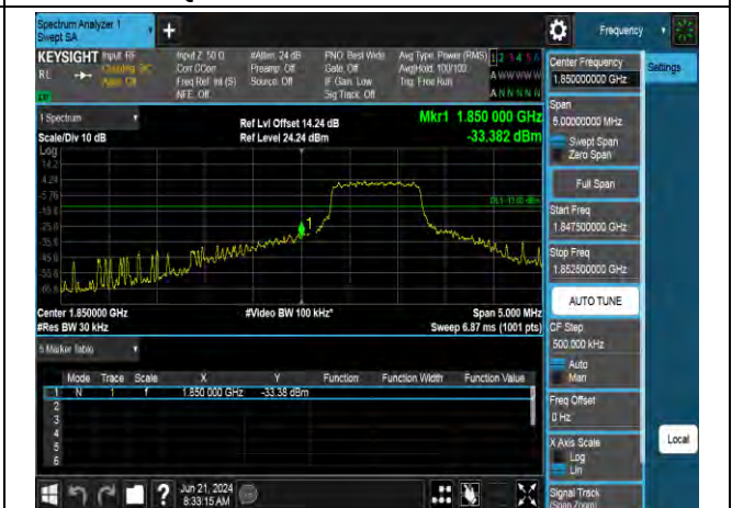
16QAM Low channel-5 RB offset 0
