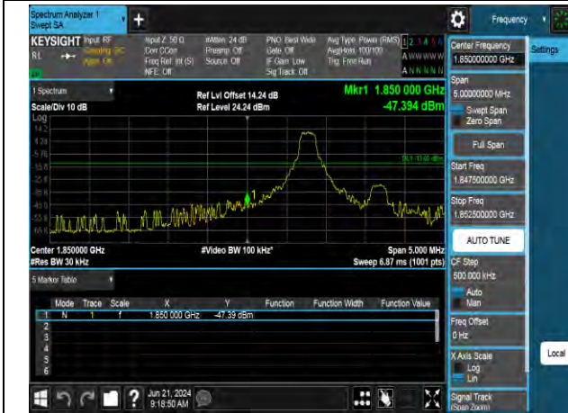
QPSK Low channel-6 RB offset 0
