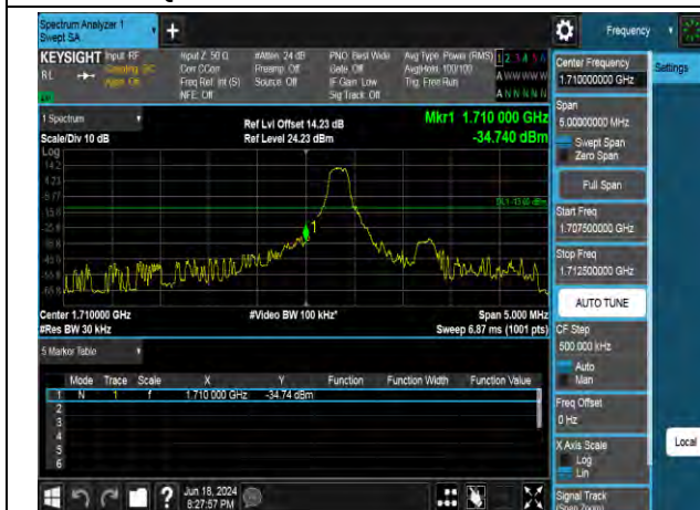
QPSK Low channel-1 RB offset 0
