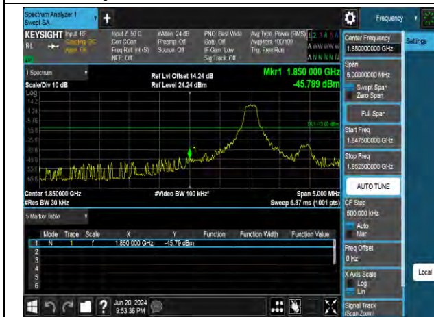
QPSK Low channel-6 RB offset 0
