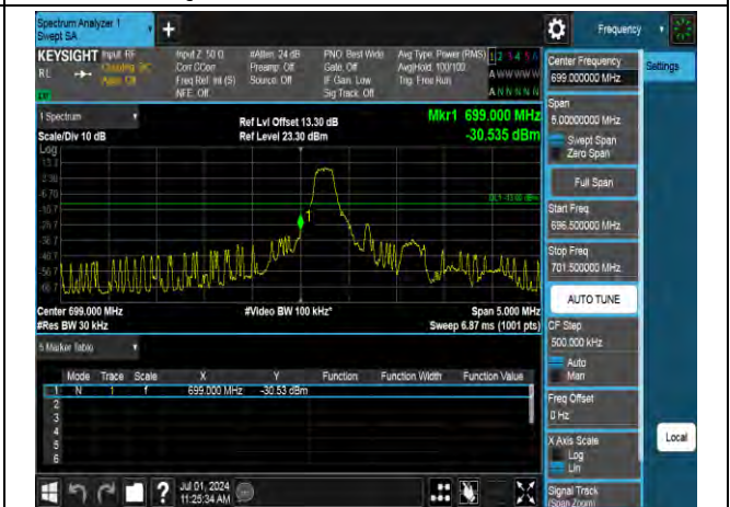
16QAM Low channel-5 RB offset 0
