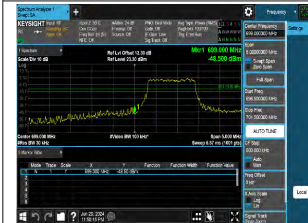
QPSK High channel-1 RB offset max
