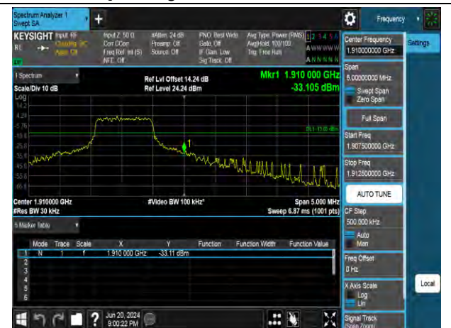
16QAM High channel-5 RB offset 0
