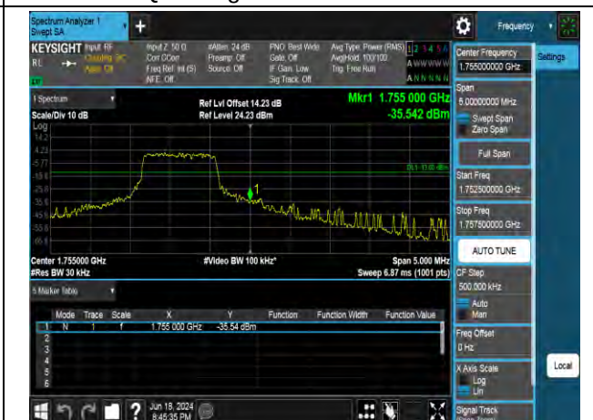
16QAM High channel-5 RB offset 0
