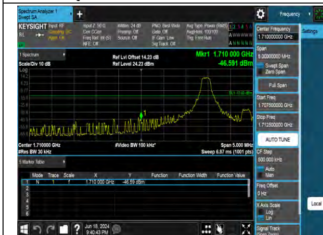
QPSK Low channel-1 RB offset 0
