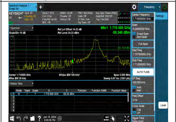
16QAM Low channel-5 RB offset 0
