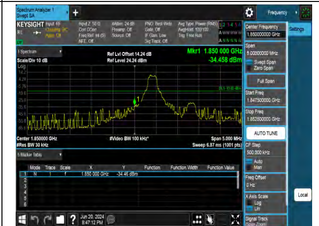
16QAM Low channel-5 RB offset 0
