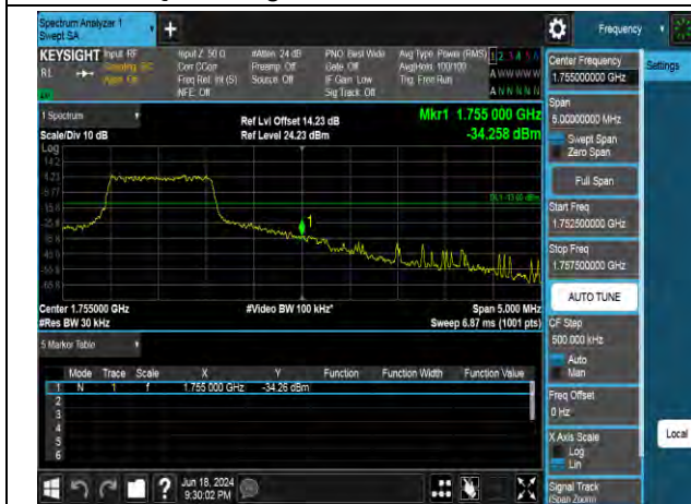
QPSK High channel-6 RB offset 0
