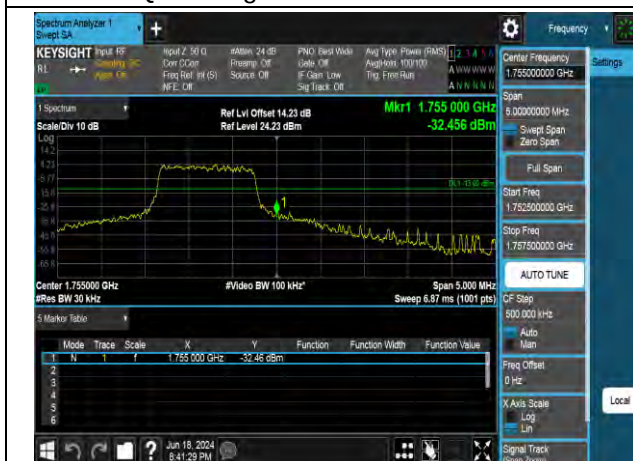
QPSK High channel-6 RB offset 0
