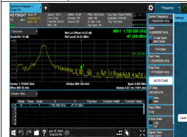
QPSK High channel-6 RB offset 0
