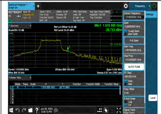
16QAM High channel-5 RB offset 0
