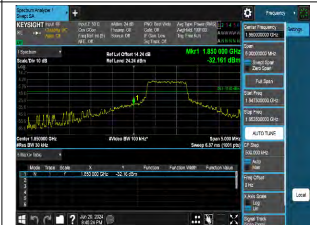
16QAM Low channel-5 RB offset 0
