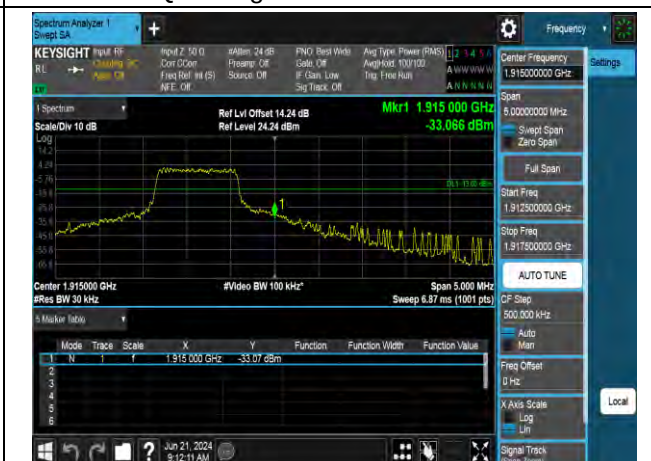
16QAM High channel-5 RB offset 0
