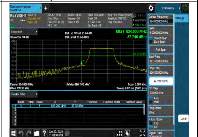
16QAM Low channel-5 RB offset 0
