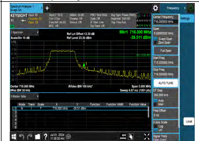
16QAM High channel-5 RB offset 0
