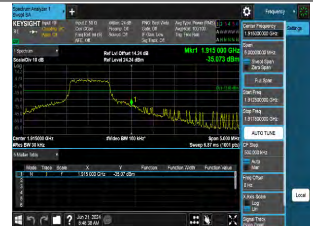
16QAM High channel-5 RB offset 0
