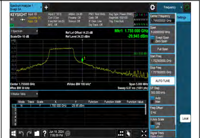
16QAM High channel-5 RB offset 0
