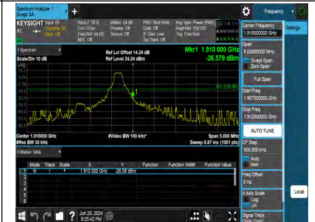
16QAM High channel-5 RB offset 0
