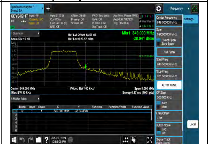
16QAM High channel-5 RB offset 0
