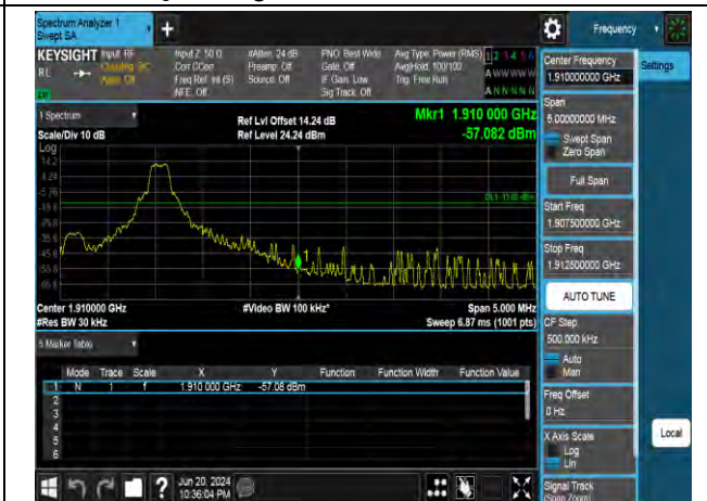
16QAM High channel-5 RB offset 0
