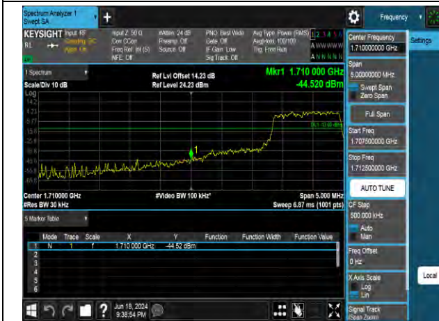
QPSK High channel-1 RB offset max
