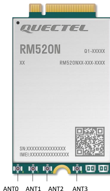
Figure 26: RM520N-GL Antenna Connectors
