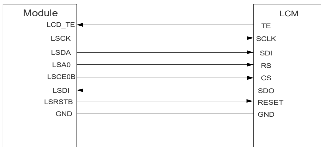
Figure 25: Reference Circuit Design for LCM Interface
