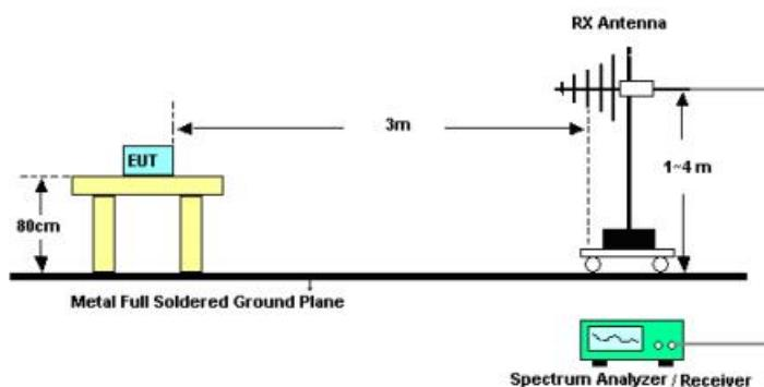
**For radiated emissions above 1GHz**
