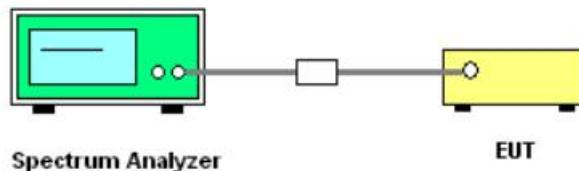
**4.3.5 Test Result of Power Spectral Density**
