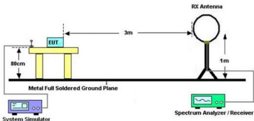
For radiated emissions from 30MHz to 1GHz
