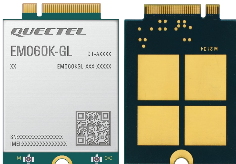
Figure 35: EM060K-GL Top and Bottom Views
