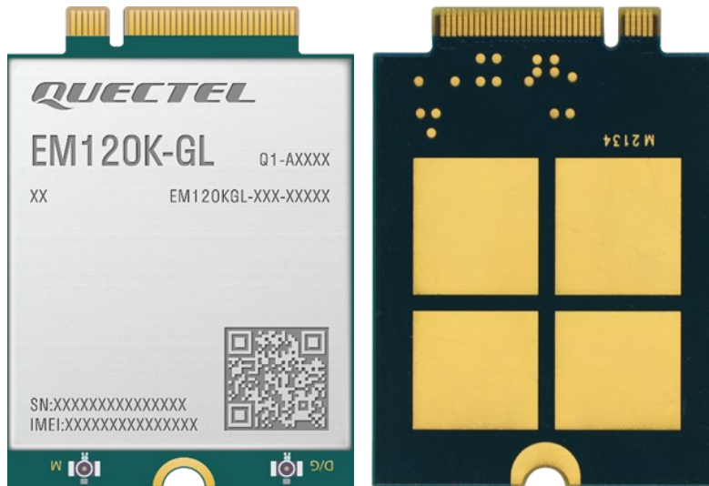
Figure 36: EM120K-GL Top and Bottom Views
