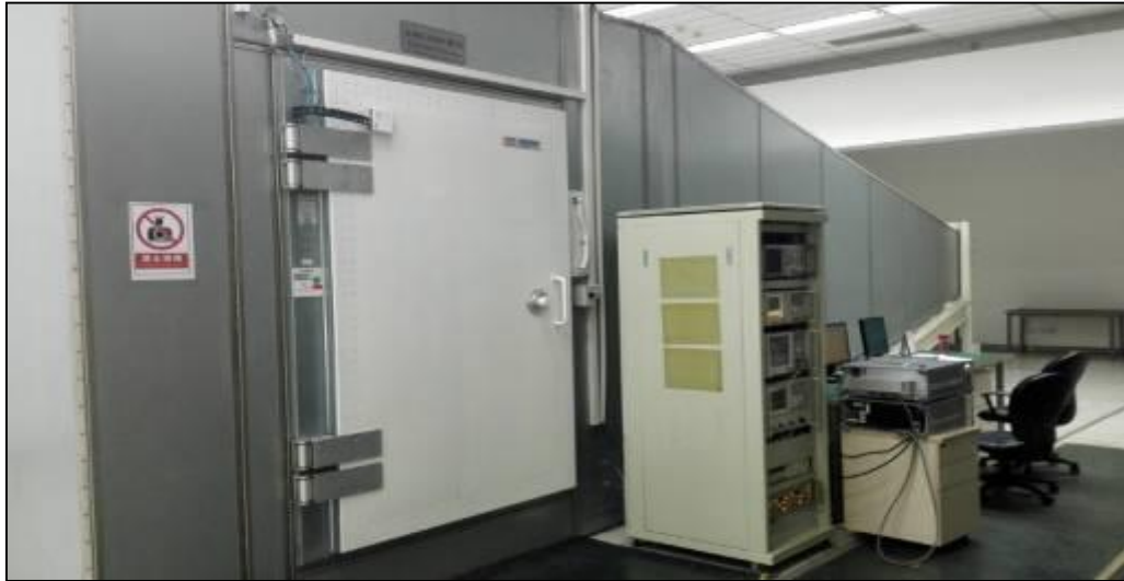
OTA Test System – ETS AMS8600
