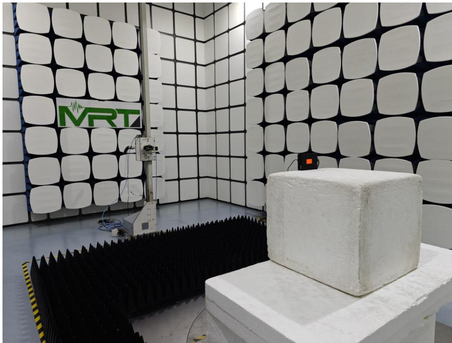
Description: Radiated Spurious Emissions Test Setup for 18GHz ~ 40GHz
