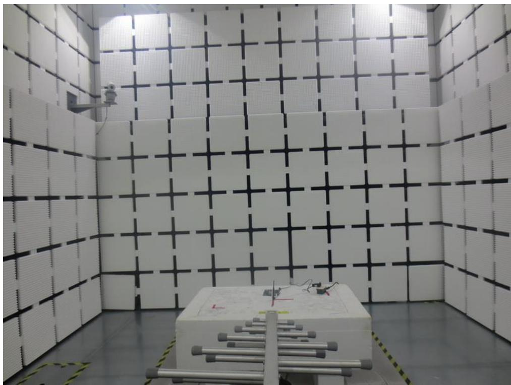
**Radiated Emissions Test Photos****Above 1 GHz**
