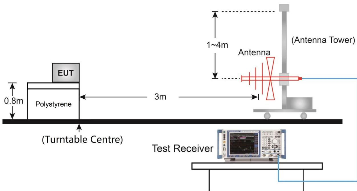
Above 1GHz Test Setup:
