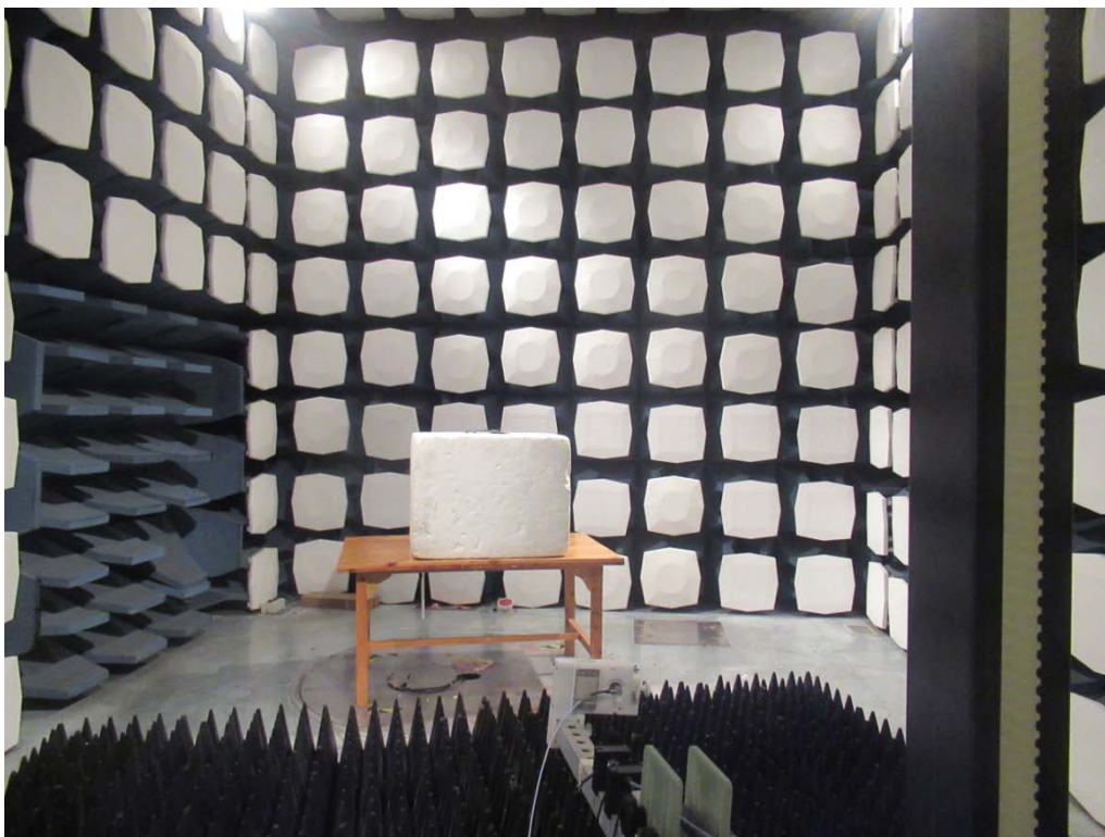
Picture 1 Radiated Emission Test Setup
