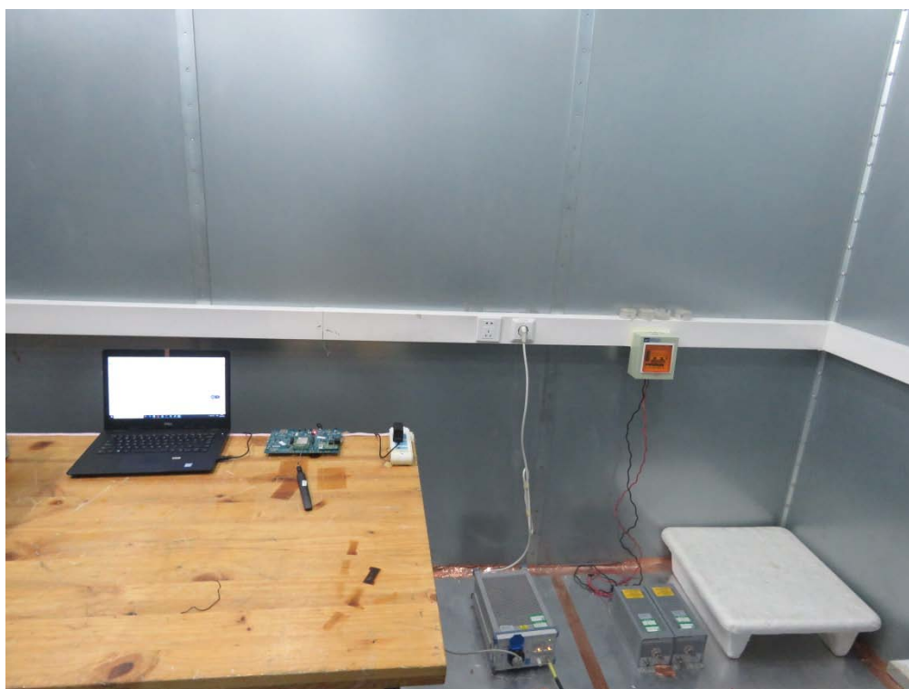
Picture 2 Conducted Emission Test Setup
